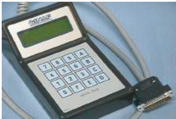
DCS-1 diagnostics unit
