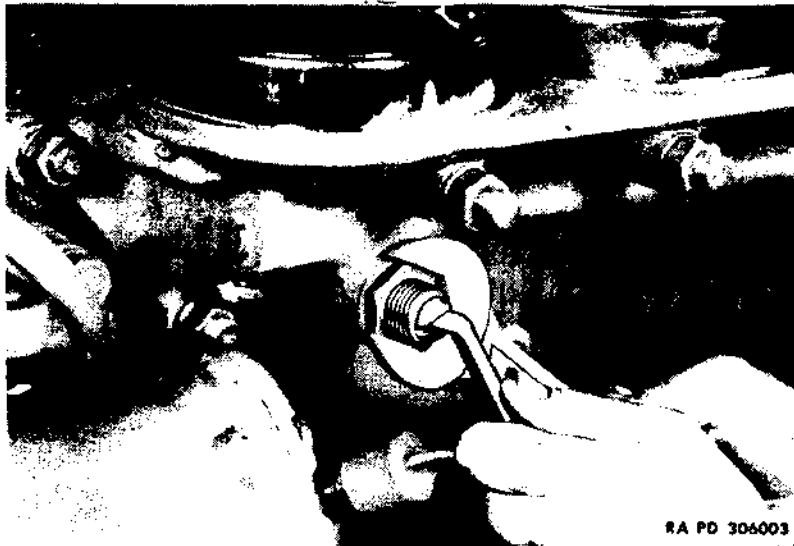
Figure 39—Adjusting Oil Pressure, Using Screwdriver 41-S-1400
