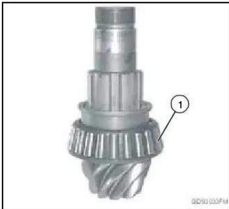
Install bearing cone (1) on pinion shaft.
