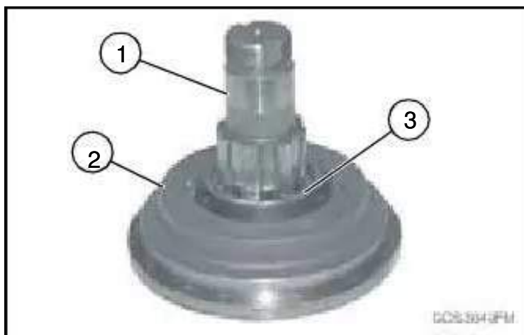
Install bearing retainer (2) on pinion shaft (1).
