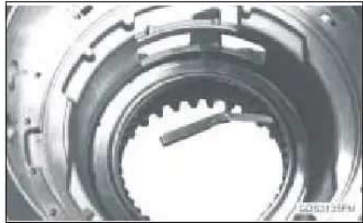
Measure plate clearance at equally spaced locations and calculate average clearance.
