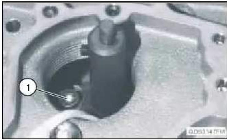
Position measurement pin (1) on pulse ring upper face and tighten set screw.
