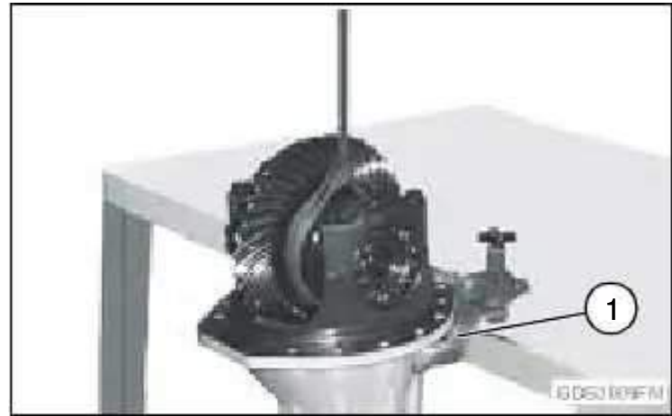
Attach D01006AA Bench Mount Fixture (1) to differential and lock in bench mount.
