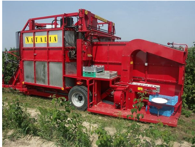
Phot. 1. Side view of "Natalia" raspberry combine harvester of Weremczuk Company [www.firmaweremczuk.com.pl]
