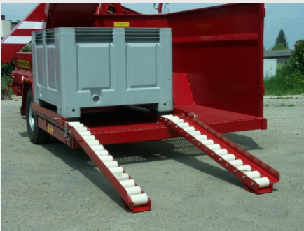
Pair of regular rollers for unloading totes
