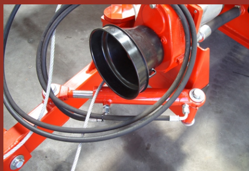
Hydraulic adjustment of draw bar position
