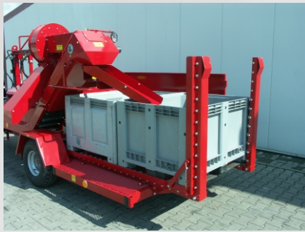
Set of equipment for placing two totes one after the other
