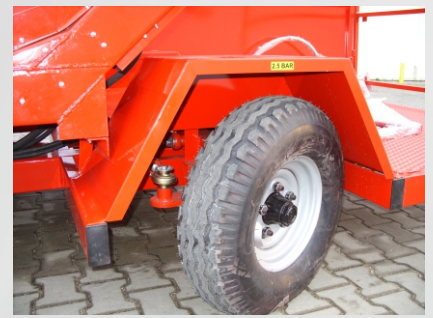
Hydraulic regulation of rear wheels turns
