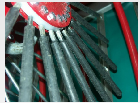
Shaking rod coated with rubber
