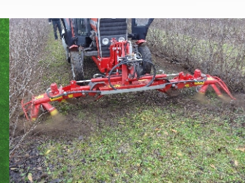
Multifunction treatment machine for orchards and plantations
