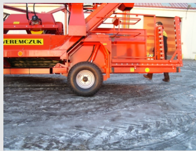
Adjustable platform wheel for work on crosswise slopes
