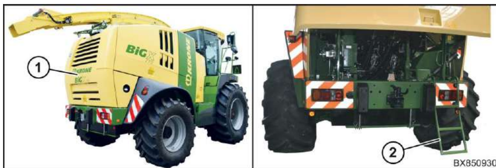
Fig. 34: Access the rear part of the engine compartment via the tailgate: Open the flap (1). • Fold down the ladder (2).
