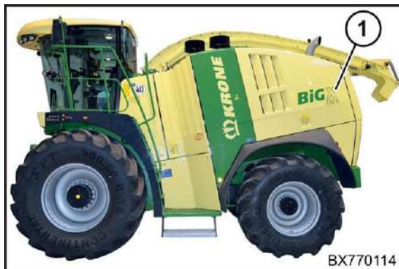
Fig. 33: The left side of the engine compartment is located under the left side flap.
