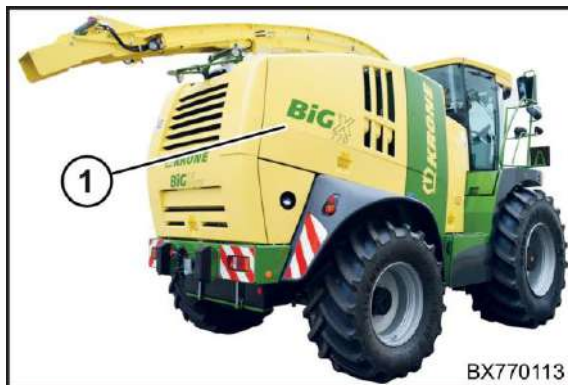
Fig. 32: The right side of the engine compartment is located under the right side flap.
