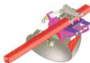
Ridging discs, spring loaded
