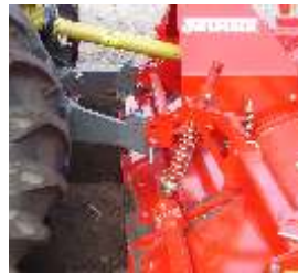
Spring loaded housing for self-cleaning
