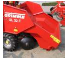
Tipping bunker for filling from trailer.
