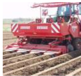
Wheels in front of the machine enable good ridge shaping
