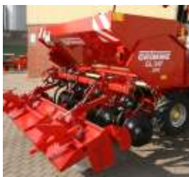
Machine with fix bunker and shaping board
