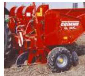
Front frame to assemble furrow opener with discs for planting in mulch rows
