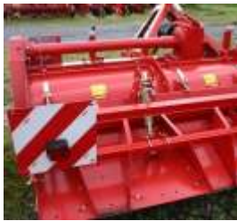
Heavy duty gear side drive
