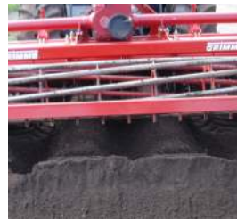
Robust tines in front of the steel roller to break the clods
