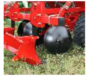
Ridging body with covering discs
