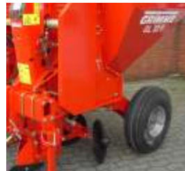
Wheels at the rear for machines with 1.000 kg bunker and moving floor bunker
