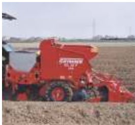
GL 32 F with fertilizer unit (option) and shaping board.
