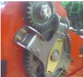
Heavy duty gear side drive
