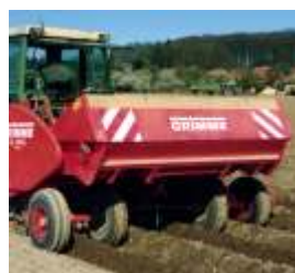
4 wheels ensure reduced ground pressure
