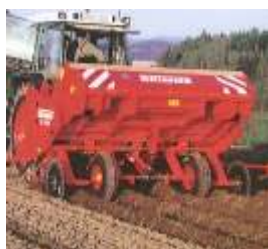
Wheels running in tractor track
