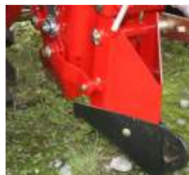
Furrow opener on parallelogram (series)
