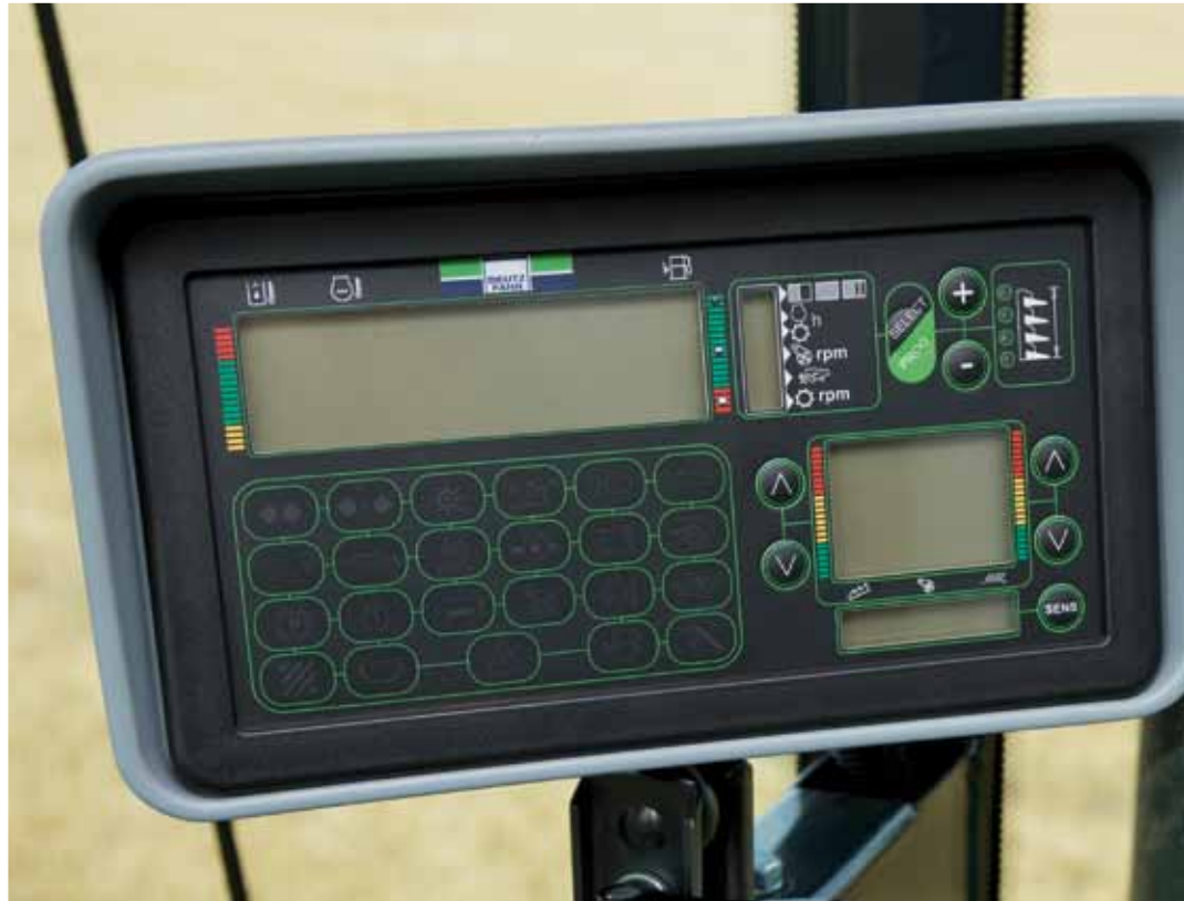
The new Combine Control Management system monitors performance of the machine in actual time.
