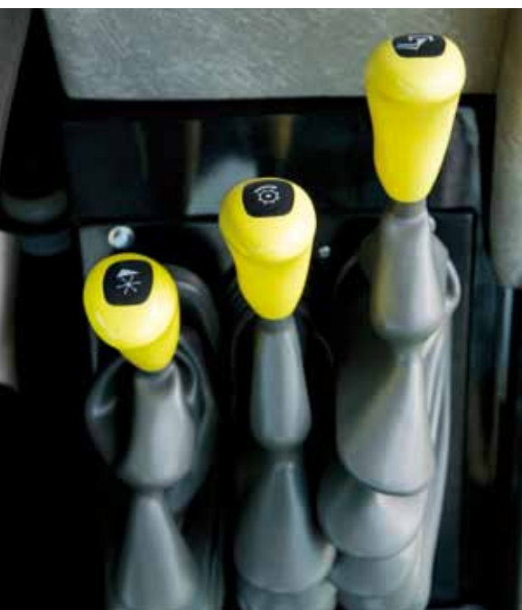
Control levers positioned on the left hand side afford optimum access to the driver seat.
