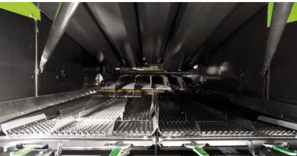
The cleaning system is top class in terms of sieving area and performance. With a cross flow fan and double drop step, the 6040 is able to deliver levels of performance hitherto unknown in this segment of the combine market.
