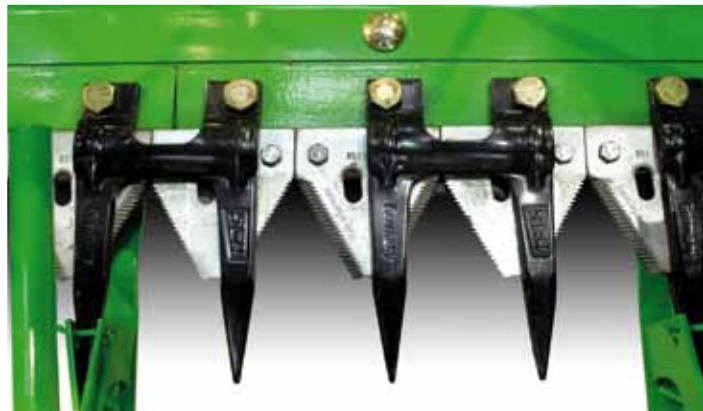
Knife sections mounted alternately edge-up and edge-down suffer less wear and ensure a Cleaner cut every time.
