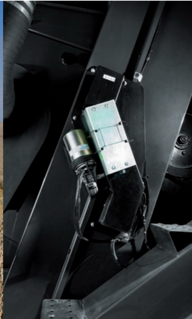
With a returns monitoring system, the operator can keep a constant eye on the capacity and productivity of the combine.
