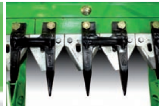
Knife sections mounted alternately edge-up and edge-down suffer less wear and ensure a clean cut every time.
