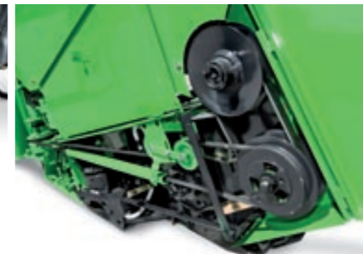
Thanks to a planetary drive and a cutting frequency of 1,220 strokes/min, the knife cuts swiftly and cleanly through the crop, whatever the harvesting conditions.
