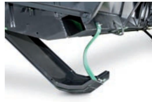
Skids ensure that the cutter bar follows the ground contours closely, instantly compensating for every ground undulation as the header advances.
