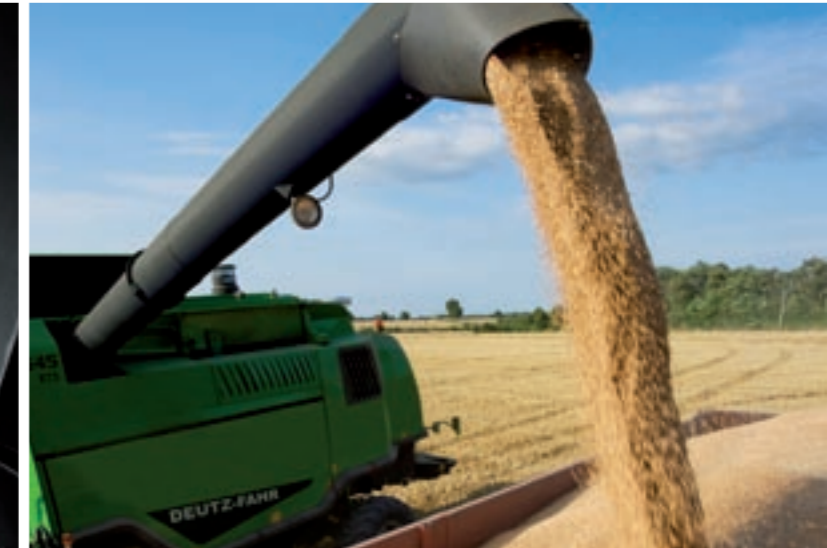
With grain discharged at a rate of 90 litres per second, the tank empties without delay and down time is cut to a minimum.
