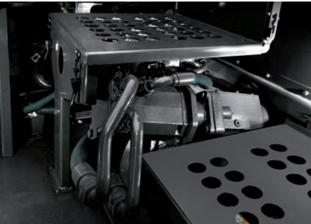
The rotor is driven by a dedicated hydrostatic system: This means that the use of drive belts can be reduced to a minimum.
