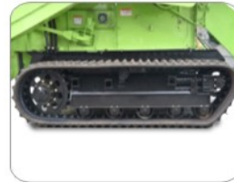
Heavy duty sprocket for long life. More width of track roller increases grip between rollers & crawlers. minimize the surface pressure
