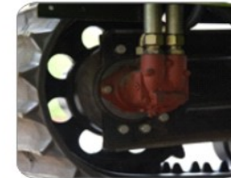
HST transmission enables to drive the machine at infinite speed ratio with maximum efficiency. front & rear movements of levers control the forward & reverse motion of machine. High quality eaton pump & hyd. motor used.
