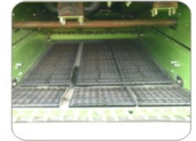
Well designed sieve section has a large cleaning area for optimum grain efficiency.
