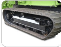
Wide crawler increases the surface contact of the machine & reduces the ground pressure. Higher level of tractive efficiency.
