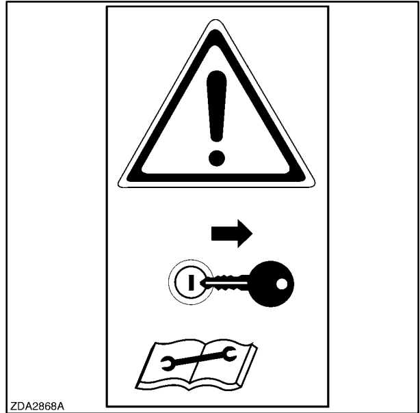
84012893 Shut off engine and remove ignition key before performing maintenance or repair work.
