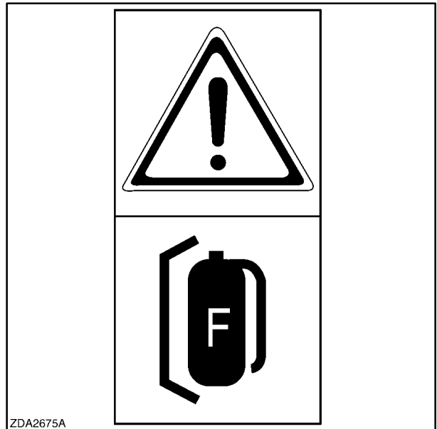
84432906 Only operate when approved fire extinguisher is installed.
