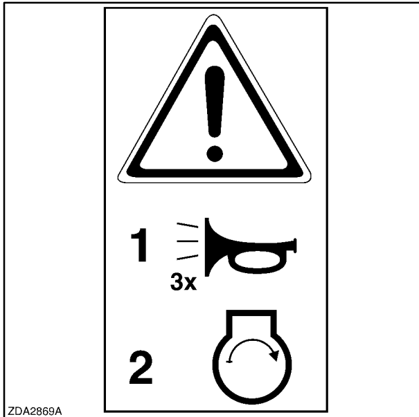
84012892 Sound the horn 3 times before starting the engine.
