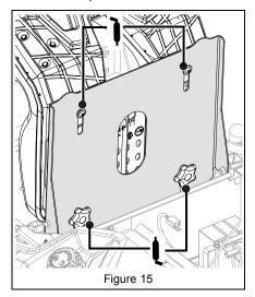
Return seat to operating position and slide seat back and forth to spread grease along tracks.
