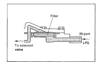
6FG/6FGF/7FG10~45/7FGF/7FG(C)U35~80 series: 2000,4~ 6FGU/6FGCU/7FG(C)U15-32 series: 2002,2~ Two types of materials are used in the filter with rubber packing for sealing in-between.
