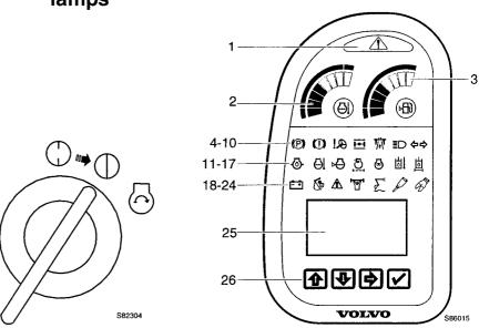
Turn the switch to running ( ( ) position, then the following control lamps should light up:
