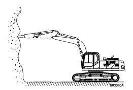
Do not strike horizontally, or in an upward direction.
