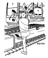
Don't use hand rail (A) of the cab door as a support. This hand rail is not strong enough to be used as a use as an access or exit hand rail. Only use this hand grip to close the door.
