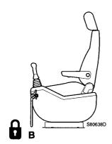
This system is used to **LOCKOUT** the attachment, swing and travel unit. Place the safety locking lever equipped on the left control console to "**Locked**" (**B**) position to lock out the hydraulic control levers.
