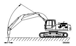
The striking direction of chisel and the direction of breaker body are deviate slightly. Therefore, adjust the bucket cylinder so that the direction of body and chisel is always the same.
