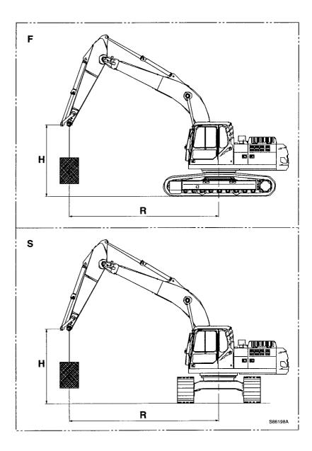
F: Lifting capacity over the front or rear of the machine
