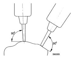
Press the chisel firmly onto the surface at a right angle as shown.
