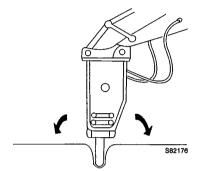
Do not bend with the chisel to make a hole in the ground.
