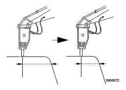
If the surface is struck repeatedly but it does not break within 1 minute, move the chisel nearer one end and strike again.
