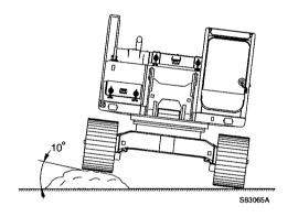
In case of traveling on uneven ground, operate the machine so as not to lean on one side more than  $10^{\circ}$ .
