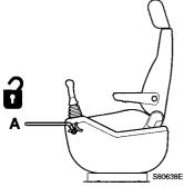
Safety locking lever "Unlocked" (A) position for working condition.
