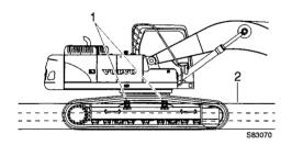
Permissible working depth in water is the center of upper rollers.
