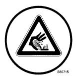
18 Warning, hot and pressurized coolant
