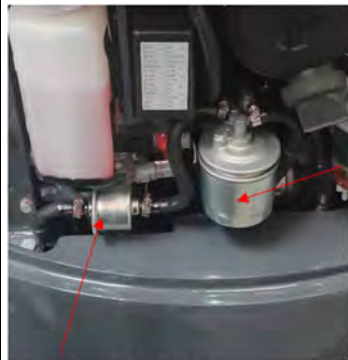
Fuel supply pump
