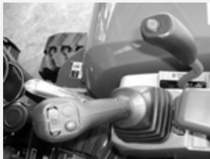
No.7 Two speed switch
