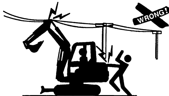
Electrical shock / electrocution
