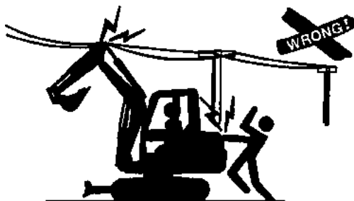
Electrical shock / electrocution
