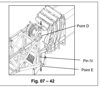
i) Remove pin V and spring-loaded pin before using jib section II;
