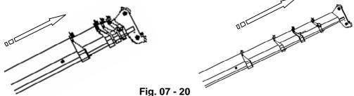
c) After the boom extends to required position, slowly tilt the pedal backward to neutral position;
