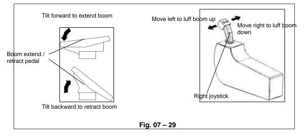
Move the right joystick and tilt the boom extend / retract pedal at a time to initiate required crane movements.
