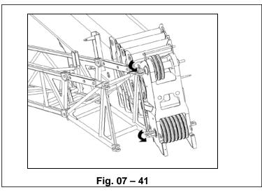
h) Connect at points D and E by inserting pin IV and guarding with load-spring pins;
