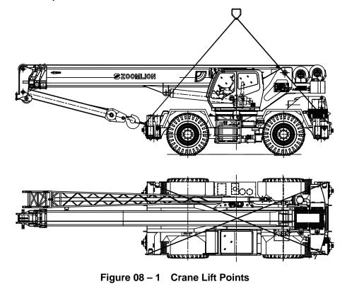
Before you lift, make sure that the slings have sufficient strength to hold the crane.
