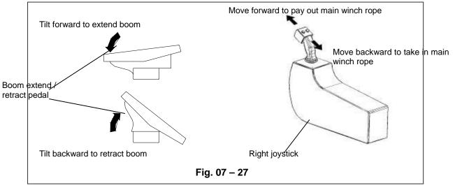
Move the right joystick and tilt the boom extend / retract pedal at a time to initiate required crane movements.
