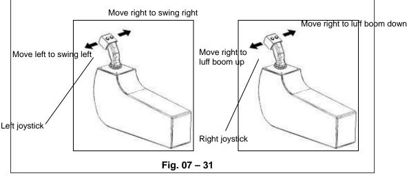
Move left and right joysticks at a time to initiate required crane movements.
