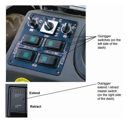
Figure 07 – 4 Outrigger Switches
