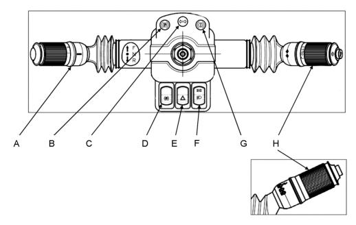
Figure 06 – 9 Combination Switches
