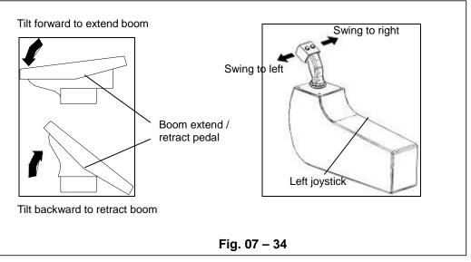
Move the left joystick and tilt the left pedal at the same time to initiate corresponding movements. See the illustration.
