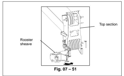
c) Auxiliary hoist rope from auxiliary winch must be laid over the upper rope guides and fed on the main boom head over sheave 3 (see Fig. 07-53) and over sheave 1 (see Fig. 07-53) of the rooster sheave. Mount the auxiliary hook and anti-two block switch. Ensure that the anti-two block switch functions correctly and all assembly connections are reliable.
