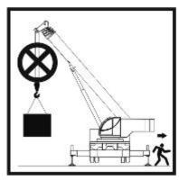
(13) When the job-site is near live power lines, you must keep a safe distance. Make sure that the dangerous area has a cover or is fenced off.
