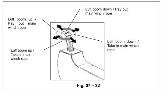
Move the right joystick between any two adjacent arrows to initiate required crane movements.
