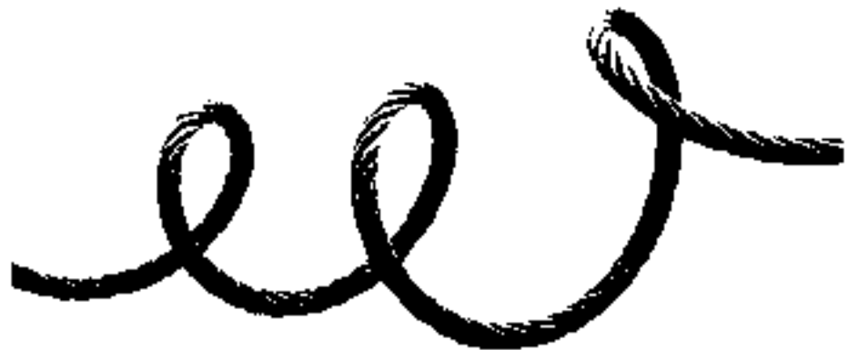
Figure 29. A corkscrewed rope ; the condition came about as a result of the rope being pulled around an object having a small diameter.
