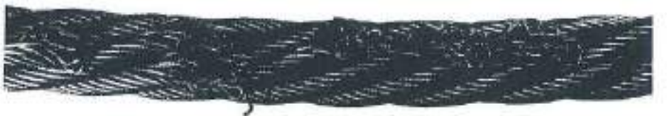
Figure 50. Here the strand wires were snagged.
