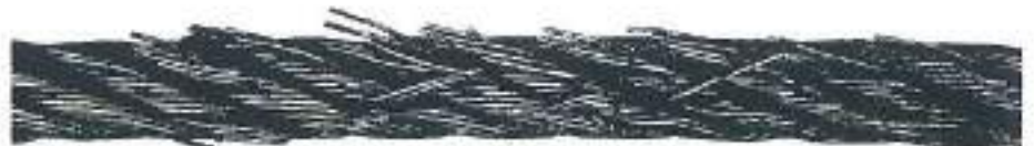
Figure 55. An illustration of valley type fatigue breaks. Flexing the rope exposes broken wires hidden in valleys between strands.
