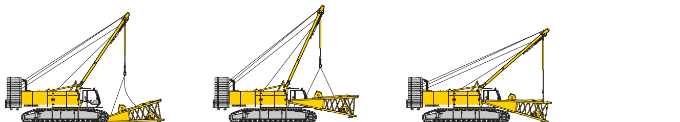
Unloading and assembly of boom foot
