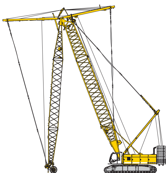
Erecting of main boom and luffing jib
