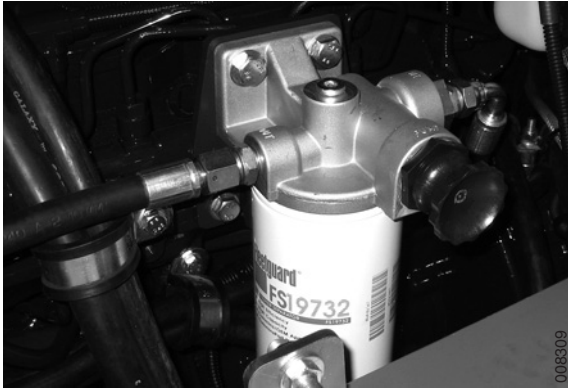
Fuel hoses on fuel filter
