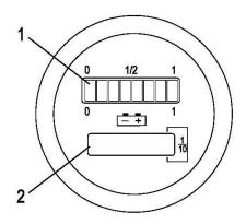
The LEDs (1) represent battery residual capacity, The LCD (2) displays the operating hours
