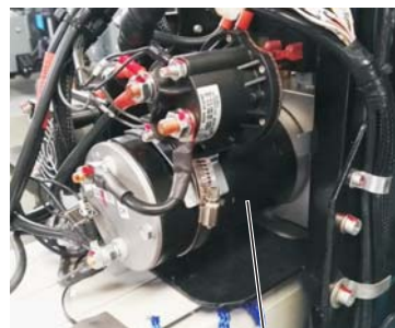
Pump and Motor Assembly
