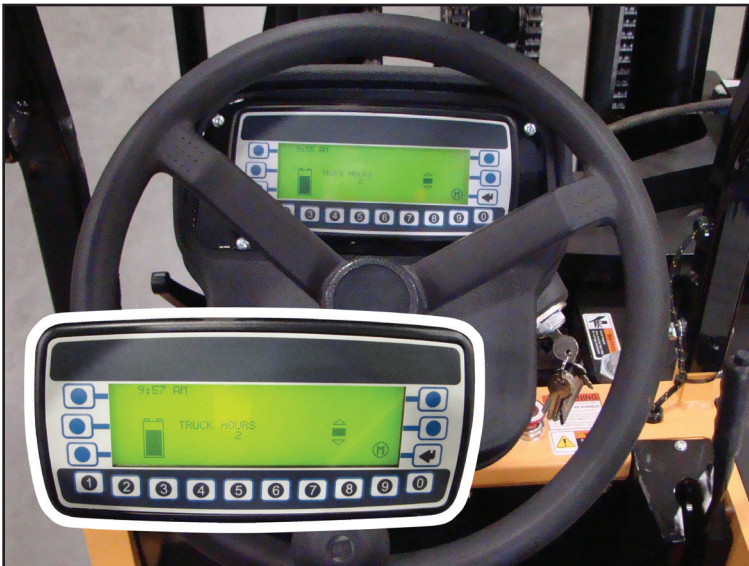
Dash Display with Full Diagnostics, Hour Meter and Battery Discharge Indicator
