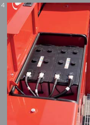
1 - 2_Engine air filter access - 3_Fuses and relays box 4_Batteries compartment - 5_Engine & transmission service bay 6_Brake system service bay
