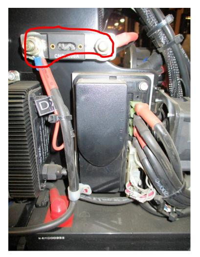
4. Check the voltage from the wire you want to check to the Controller negative (red circled).
