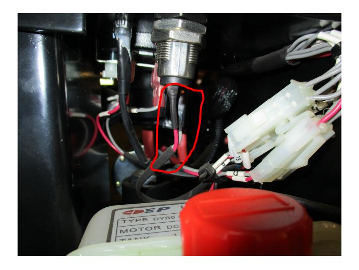
Check if connectors are loose or burned (such as the 2 pin connectors on the Main Contact). Ensure the parts are properly tightened.
