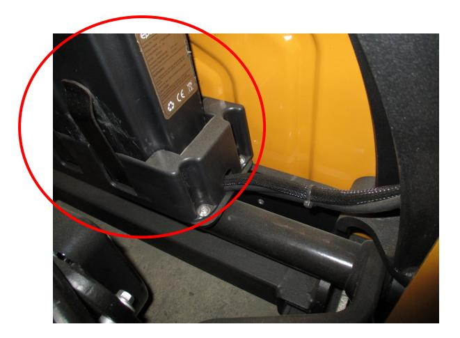
Check the no load battery voltage for every battery.
