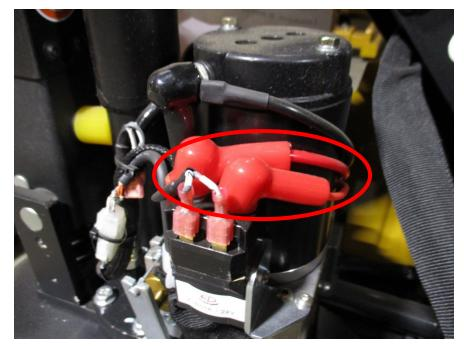
Check the connection points of the motor cables, and controller cables. Check the cable terminals for burn marks. Check if hardware is loose or burned. Ensure connections re tightened properly.
