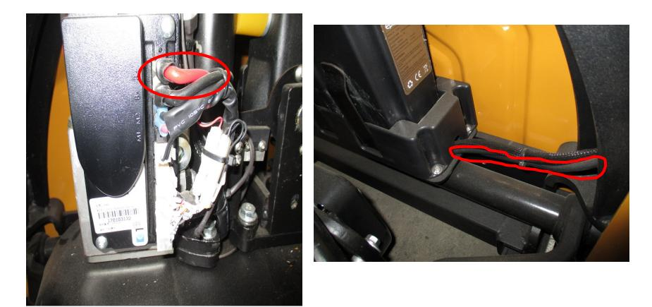
Check the Connectors between Battery and truck to see if they fit loose or are burned (Concentrate on the inside of the connector). If they do not fit correctly, replace cable lugs and/or connector housing to correct the issue.
