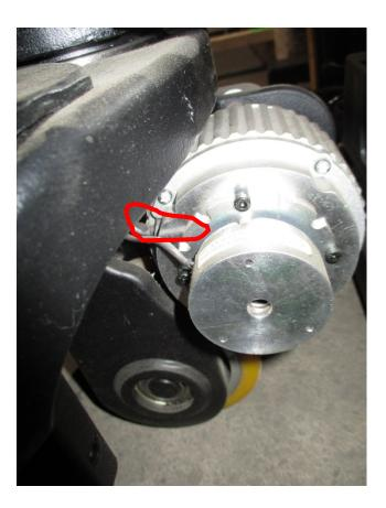
2. Check if cables are opened or shorted. A shorted cable means the cable jacketing is damaged and it is shorting to another cable or it is in contact with a metal object like the frame. An open cable means one of the inside metal wires are cut/damaged. If you are not sure, pleasure measure the resistance of the individual wire or cable. If the resistance is more than 1 ohm, it is open.
