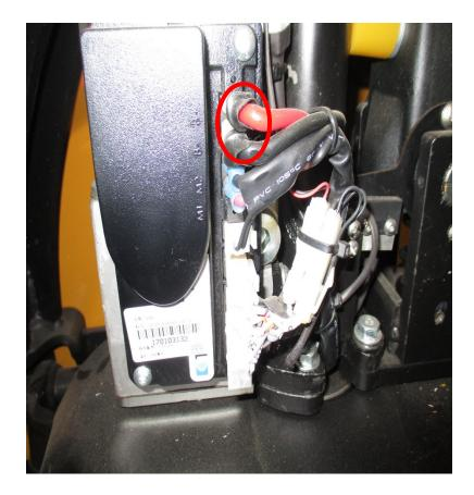
Check the connections between Controller wires and switches/sensors. Ensure wires are not cut or damaged.
