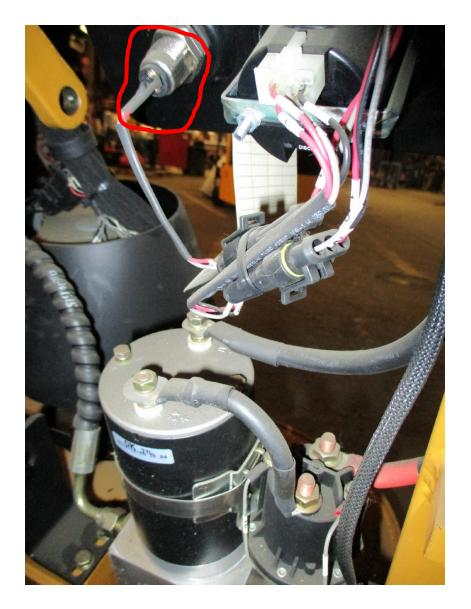
Check if connectors are loose or burned (such as the 2 pin connectors on the Main Contact). Ensure the parts are properly tightened.
