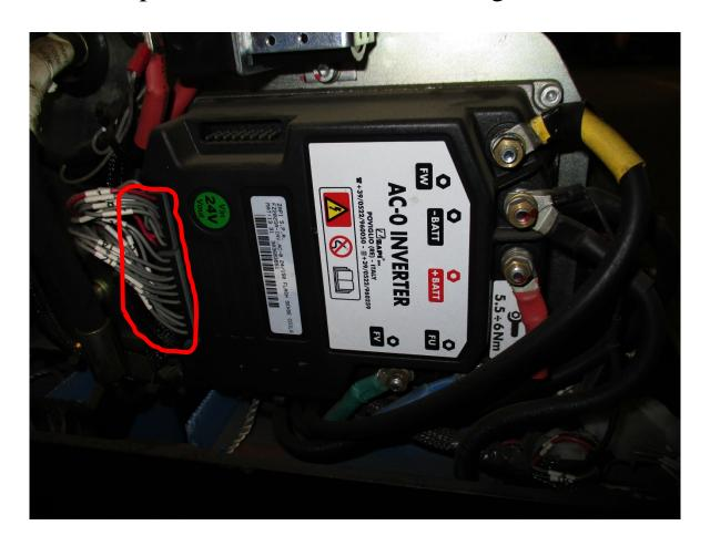
Check the connections between Controller wires and switches/sensors. Ensure wires are not cut or damaged.
