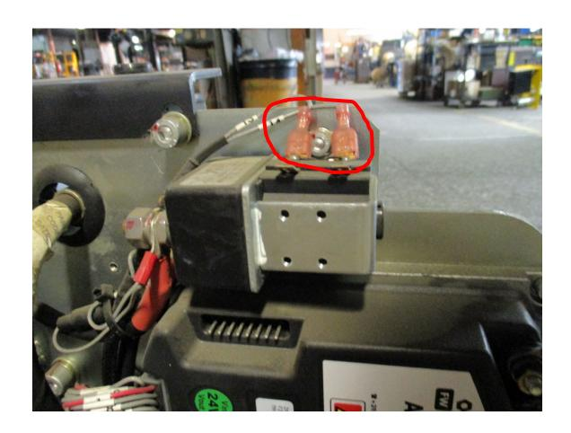
3. Check if cables are opened or shorted. A shorted cable means the cable jacketing is damaged and it is shorting to another cable or it is in contact with a metal object like the frame. An open cable means one of the inside metal wires are cut/damaged. If you are not sure, pleasure measure the resistance of the individual wire or cable. If the resistance is more than 1 ohm, it is open
