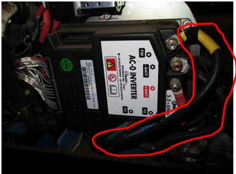
Check the connection points of the motor cables, and controller cables. Check the cable terminals for burn marks. Check if hardware is loose or burned. Ensure connections are tightened properly.
