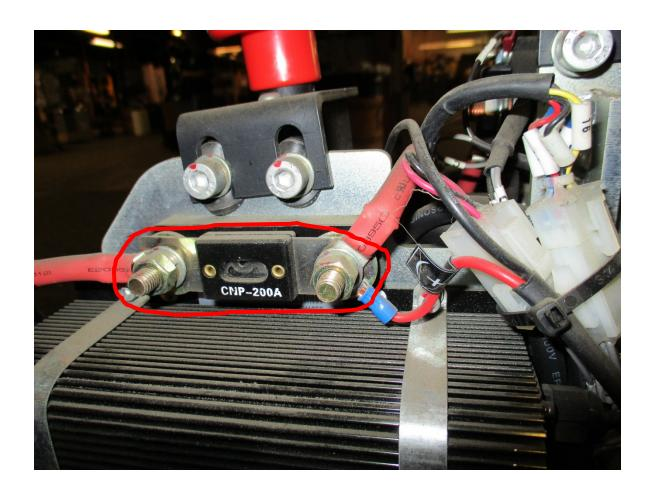
4. Check the voltage from the wire you want to check to the Controller negative (red circled).
