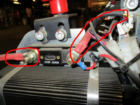
Check the Connectors between Battery and truck to see if they fit loose or are burned (Concentrate on the inside of the connector). If they do not fit correctly, replace cable lugs and/or connector housing to correct the issue.
