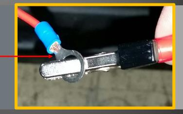
4. Secure the Negative Meter Lead to the Stud that you removed the wire from. Your Volt OHM Meter is now in Series between the Charger and the power cable.
