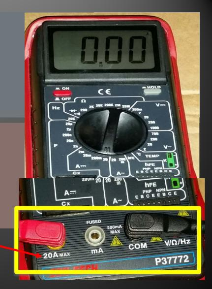
3. Secure the Positive meter lead with an alligator clip to the Positive Red Charger wire you removed. –
