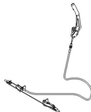
Fig.2-4 Parking brake device
