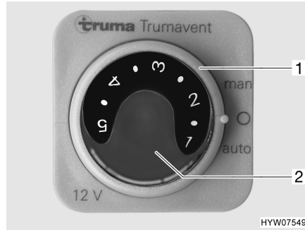
Fig. 76 Operating switch for circulation fan (12 V)
