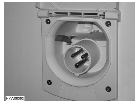
Fig. 58 240 V connection on vehicle
