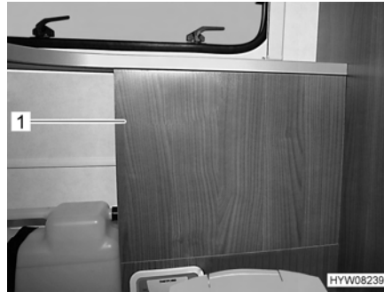
Fig. 91 Panel for water canister
