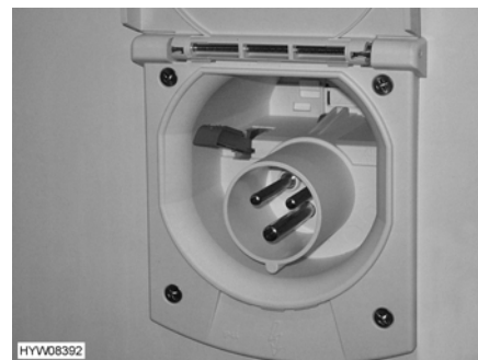
Fig. 58 240 V connection on vehicle
