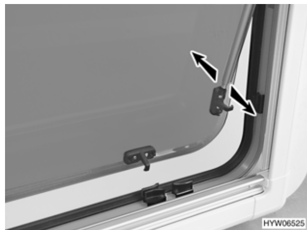
Fig. 42 Hinged window, telescopic rod (variant 2)
