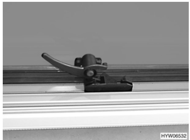
Fig. 44 Hinged window in the "continuous ventilation" position (variant 2)
