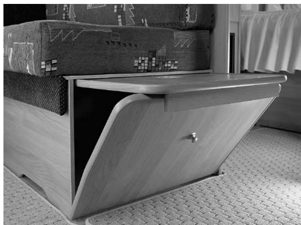
Bed expansion for vehicles with rear seat group.
