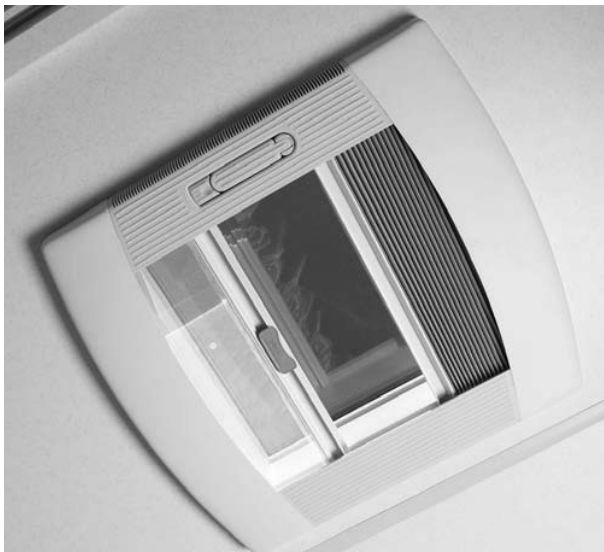
Thermal roof bonnet in bedroom
