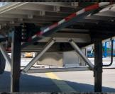
Aluminum landing gear braces are lighter than steel and withstand the beating from rocks and road debris.
