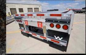
Roadbrute and Premier flatbeds are standard with an extruded aluminum rear end with aluminum R.I.G. (Steel R.I.G. is optional on the Roadbrute.)
