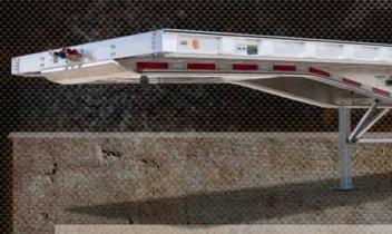
The Premier AF-1080 All Aluminum flatbed has a base weight of approximately 8,000 lbs. on a typical 48 ft. unit and a 23" main beam depth. The trailer features one-piece aluminum flanges and sections without any splices and its load capacity rating is among the highest in the industry.
