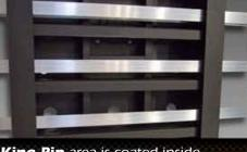
The **King Pin** area is coated inside and out with Corsol to seriously reduce corrosion in this critical area. The design is also void of any corrosion harboring tubes plus it makes use of the full-width aluminum crossbars which add strength while reducing the trailer's overall weight.
