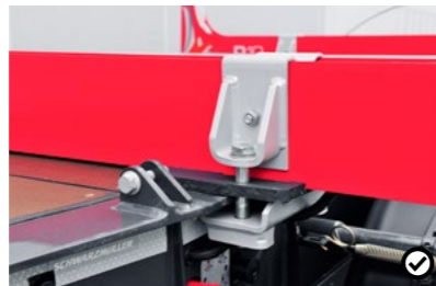
1 Mounted fitted timber-stad These are attached to the vehicle by clamp fastening and therefore horizontally-adjustable as required. They serve to ensure secure transportation of the cargo (logs).
