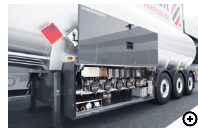
F Solid fittings cabinet Made of aluminium with product-collecting channel on both sides. Left: gas return connection and API filling couplings. Right: individual drains.
