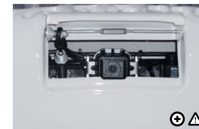
S Rear view camera This offers added safety for reversing; the camera cap opens pneumatically.
