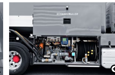
I Pump and measurement system Available as an alternative to the electronic dipstick for empty and full hose delivery.
