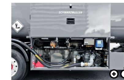
J Gravity measurement system Instead of an electronic dipstick, there is the option of a PD-meter measurement system for discharging by gravity.
