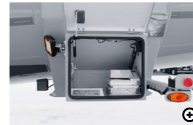
7 Fibreglass-reinforced plastic printer cabinet
