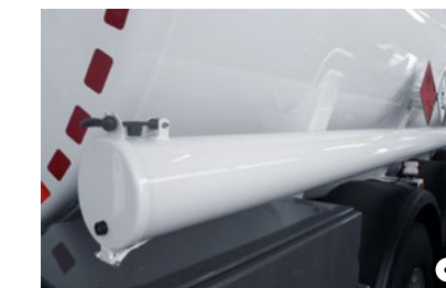
G Hose storage The vehicle can be equipped with an additional 7.5m long hose storage.
