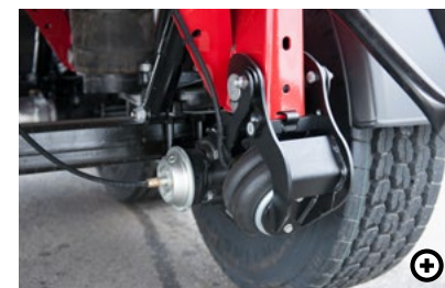
C Lifting axle Lifting axle reduce tyre wear by means of automatic axle raising during empty runs. These also serve as a starting aid.
