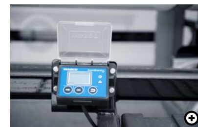
D SmartBoard The SmartBoard from Wabco displays various vehicle data on an integrated display.
