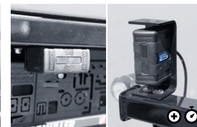
U Wabco tailGUARD™ Safety system with three sensors that combines rear-area monitoring with automatic braking.
