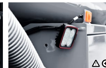
L Working lights The LED lights provide extra lighting during the loading and unloading process.
