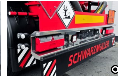
N Stainless-steel under-run protection High-shine stainless-steel under-run protection.
