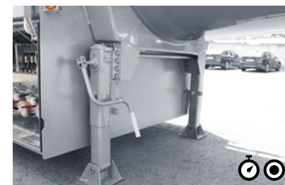
B Landing legs Schwarz Müller offers a choice of landing legs: either in the form of a steel or aluminium crank-handle leg or steel or aluminium support legs.
