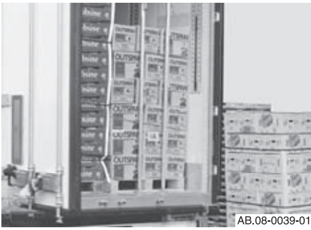
Flexible load securing gear at the rear with telescopic clamping bars (example)
