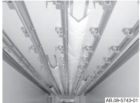
European meat hanging system for clockwise meat hooks (the hooks rotate clockwise from the rail)
