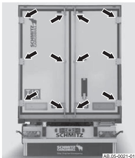
Positions of the screws on the rear door frame: Locking elements and hinges
