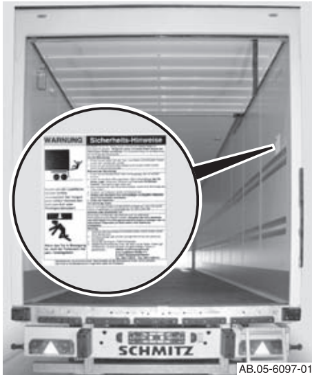
"Roller door" safety notice
