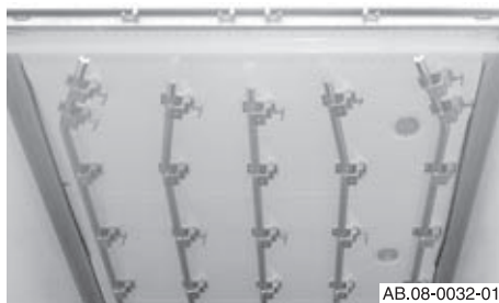
Danish meat hanging system for anticlockwise meat hooks (the hooks rotate anticlockwise from the rail)
