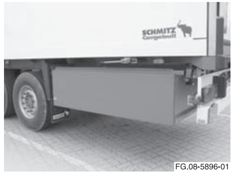
Pallet boxes with bracket lock (behind the axle assembly) FP 25 and FP 45/FP 60
