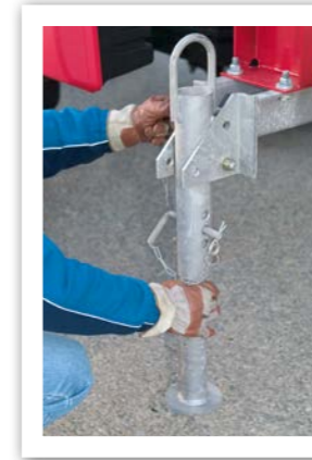
Rear landing leg. Additional landing legs at the rear with bolt locking serve as supports for the vehicle in case of loading/unloading from the rear. Thus the trailer connection is prevented from damage.
