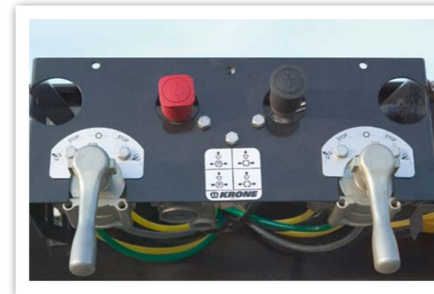
Lateral control levers. Control levers located on one side for safe operation during swap body movement.
