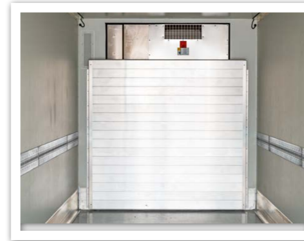
Solid evaporator guard. Added protection: the evaporator guard is formed from aluminium profiles.
