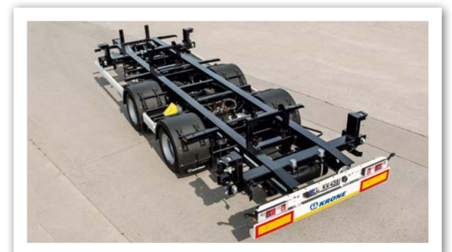
The Multi Box Carrier is fitted with flexible twist locks. It is designed with a ground clearance of 970 to 1320 mm (alternatively 920 - 1270 mm).
