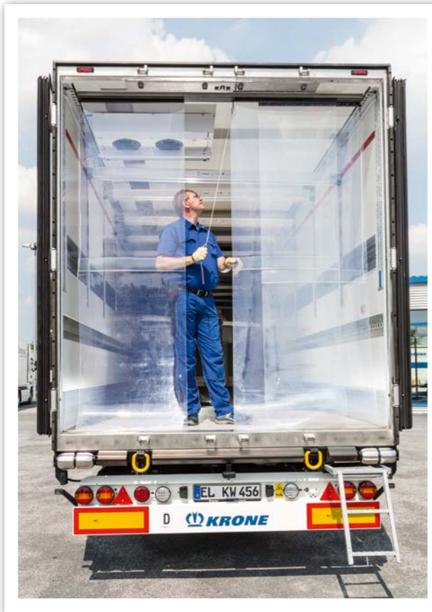
Strip curtain. The insulation strip curtain is in three parts.
