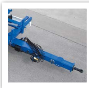
Bolted drawbar. The tow bar and coupling eye is bolted to the chassis which, in the event of damage, reduces replacement cost.
