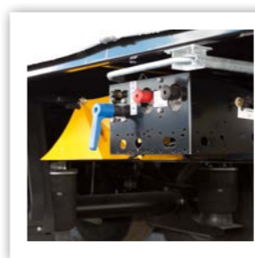
Protected valves. The setting valves are well protected behind the axle assembly. The wheel chocks, too, are always at hand there.
