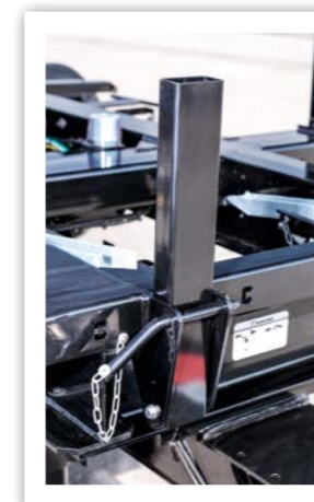
Solid stops. Folding solid stops allow accurate swap operations.
