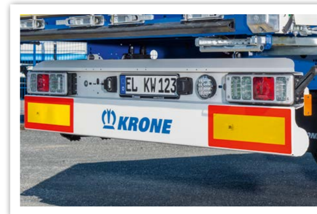
Underrun protection and light panels as individual components. The separate and screwed-on execution of the components allows a quick and smooth replacement.
