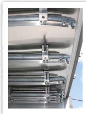
Meat-Hang-execution. Various models for suspension of meat are available that comply with country-specific requirements. Available are meat suspension rails with 60 mm or 45 mm diameter. Hook catch and Hook separation guard as standard equipment. On request, with hook parking rail or rack.
