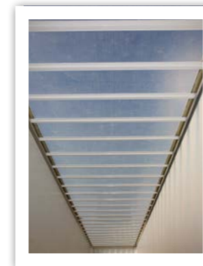
Translucent plastic roof. Better vision during loading and unloading work thanks to the translucent plastic roof. Segments of this design can also be optionally installed.
