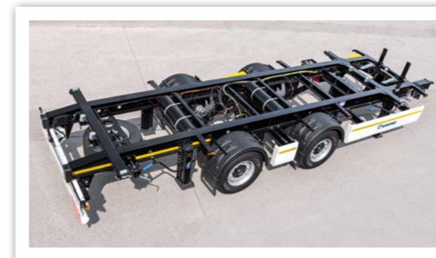
The Profi Box Carrier B10 with centre axles carries swap container sizes C782 - with an optional pallet stop - and sizes C715 and C745. It is designed with a ground clearance of 1,070 mm to 1,320 mm.
