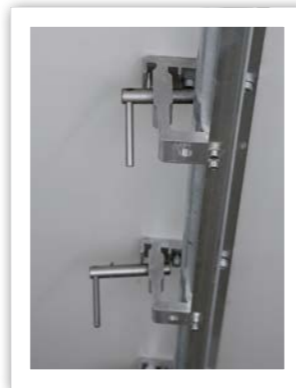
Meat-Hang-execution. Various models for suspension of meat are available that comply with country-specific requirements. Available are meat suspension rails with 60 mm or 45 mm diameter. Hook catch and Hook separation guard as standard equipment. On request, with hook parking rail or rack.
