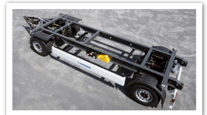
The Profi Box Carrier B7 is built for transporting high-volume swap bodies. It is designed with a ground clearance of 1,020 to 1,320 mm.
