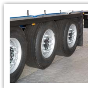
Effective spray protection. The wheel arches and the mudguards are provided with spray suppression as standard.
