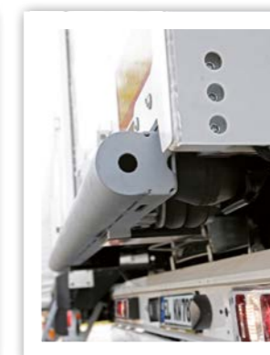
Compression buffer. Tough to break: that is the compression buffer. Extremely robust impact protection of steel at the tail end with impact-absorbing rubber blocks for damping docking forces. (Optional)
