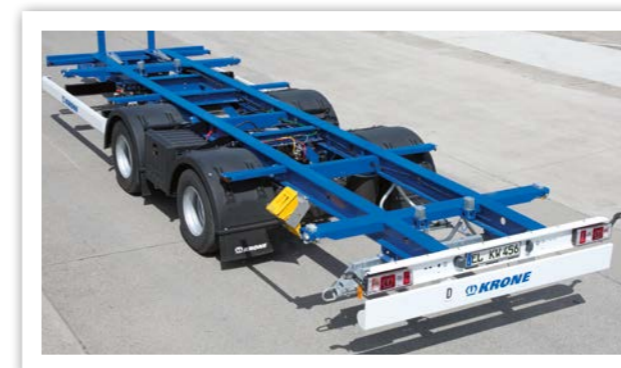
The Mega Box Carrier in central-axle design is built for transporting high-volume swap bodies. It is designed with a ground clearance of 1,020 to 1,320 mm.
