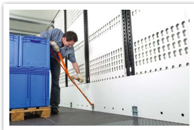
Versatile load securing. Besides key hole profiles there are also lashing rings for load securing integrated in the side kick strips, available.
