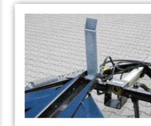
Equipment of central axle trailers. The central axle trailer is well suited for high-volume and standard swap bodies with height-adjustable twist locks and fold-away spacers, both equipped with turning mechanism.
