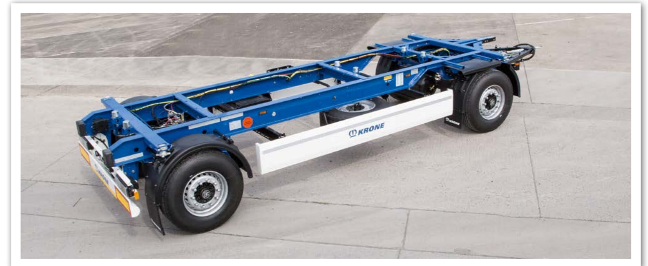
The Profi Box Carrier B9 is designed for a parking level of 1,220 and 1,320 mm, which is standard for swap body transport.
