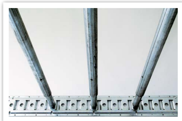
Variable interior equipment. The steel coffer model of the Dry Liner is equipped with keyhole plates as standard. The plywood series features attached strapping rails.
