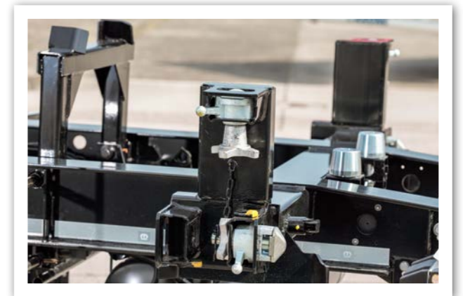
Equipment of central axle trailers. The central axle trailer is well suited for high-volume and standard swap bodies with height-adjustable twist locks and fold-away spacers, both equipped with turning mechanism.
