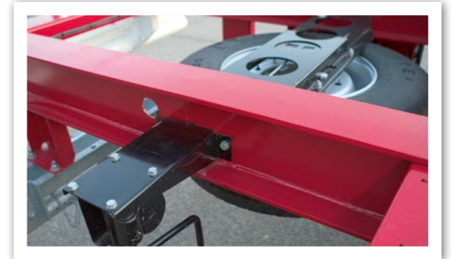
Spare wheel holder. Swap trailers for high-volume transport are equipped with a winch-type spare wheel holder.
