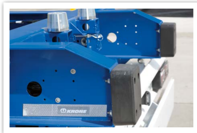
Sophisticated swap solution. Slanted rear ends on the longitudinal beams allow easy mounting on uneven ground.
