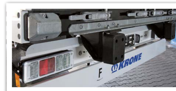
Compression buffer. Tough to break: that is the compression buffer. Extremely robust impact protection of steel at the tail end with impact-absorbing rubber blocks for damping docking forces. (Optional)
