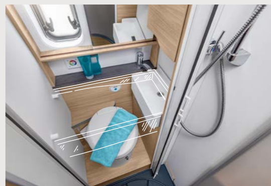
BOXSTAR 630 FREEWAY. The hand basin in the open bath can be converted into a large washbasin in a few easy steps.
