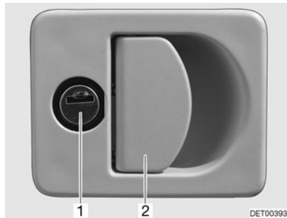
Fig. 13 Flap lock with recessed handle
