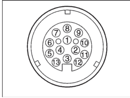
Fig. 101 Top view on socket towing vehicle (thirteen-pin system Jaeger to DIN EN 1648-1)
