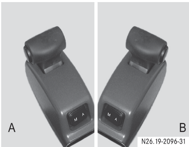
Telligent ® automatic gearshift system, see page 73
