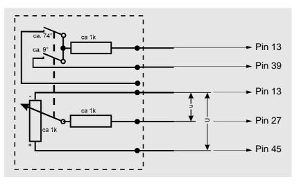
U = Reference voltage, approx. 5 V from the EDC control unit u =Setpoint
