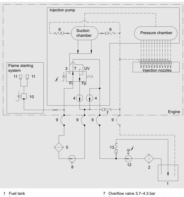
Fuel circuit diagram – engine shutoff using EHAB
