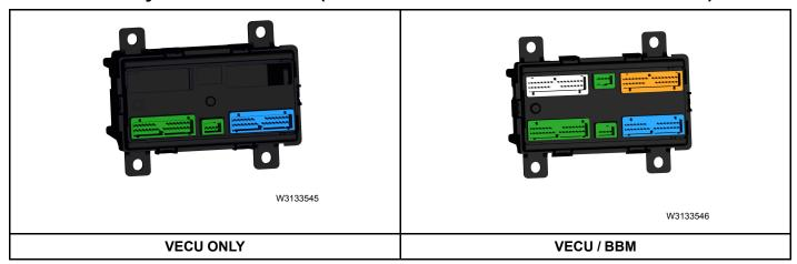
**Note:** BBM will have the white and orange connector plug and the VECU will have the blue and green connector.
