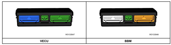
**Note:** BBM will have the white and orange connector plug and the VECU will have the blue and green connector.
