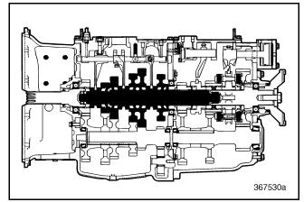
Figure 396 — Front Mainshaft Component Locator (T313L/T318L Shown)
