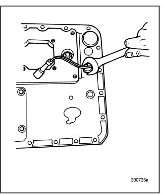
Figure 486 — Installing Reverse Light Switch
