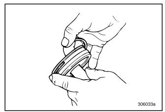
Figure 183 — Removing Wiper Ring from Piston Groove
