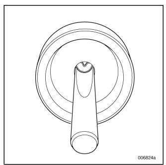
Figure 448 — Inserting Teflon<sup>®</sup> Seal Installer/Sizer (Tool No. J 47358)
