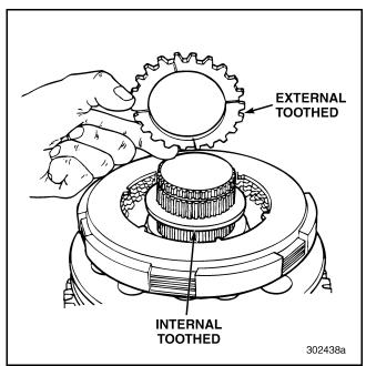
Figure 390 — Installing External-Toothed Thrust Washer (T313L21/T318L21 Shown)
