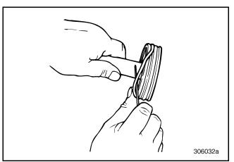
Figure 450 — Installing O-Ring in Second/Lower Groove on Piston
