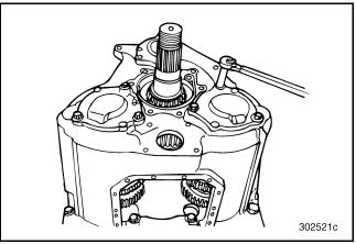
Figure 559 — Tightening Rear Countershaft Bearing Cover Capscrews (T313L21/T318L21 Shown)
