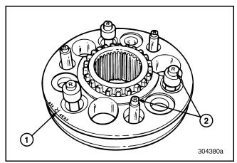
Figure 359 — Synchronizer Pins and Sliding Clutch Temporarily Assembled to Show "R" Marks
