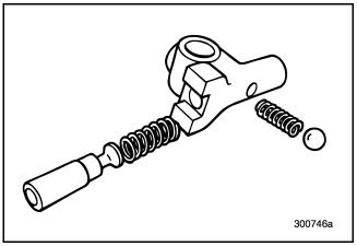
Figure 499 — Assembling Lo/Reverse Shifter
