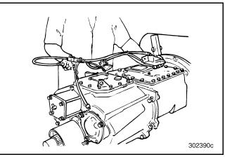
Figure 64 — Removing Air Lines and Valves
