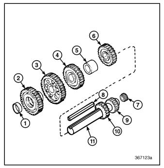
Figure 599 — Exploded View of Front Countershaft
