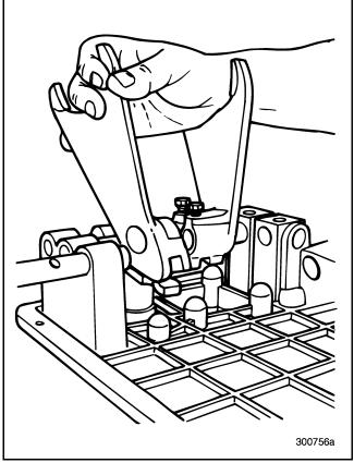
Figure 498 — Installing Third/Fourth Shift Fork
