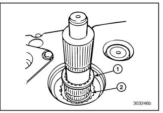
Figure 108 — Removing Internal-Toothed Thrust Washer and Snap Ring (T313L/T318L Shown)
