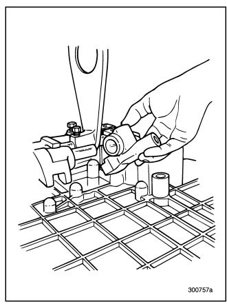
Figure 139 — Removing Lo/Reverse Shifter
