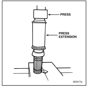
Figure 349 — Pressing Bearing onto Output Shaft
