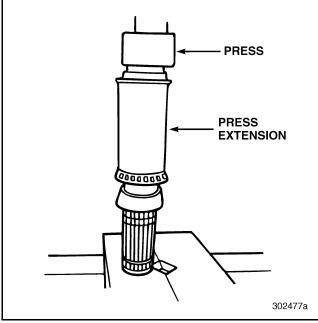
Figure 367 — Pressing Bearing onto Output Shaft (T313L21/T318L21 Shown)
