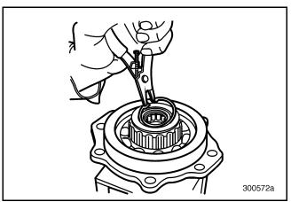
Figure 433 — Installing Spigot Bearing and Snap Ring
