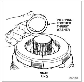
Figure 244 — Removing Internal-Toothed Thrust Washer and Snap Ring (T313L21/T318L21 Shown)
