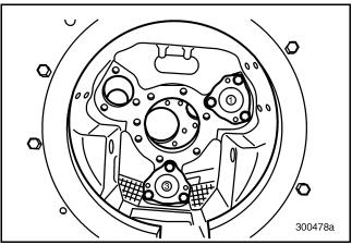
Figure 125 — Remaining No. 1 and No. 3 Front Countershaft Bearing Covers
