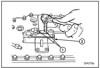
Figure 580 — Tightening Remaining Range Shift Valve Screws
