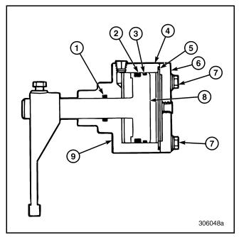
Figure 605 — Cutaway View of Two-Position Range Shift Cylinder
