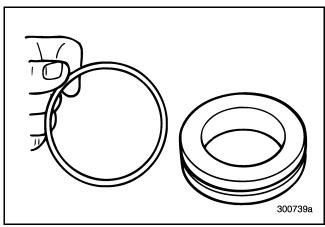
Figure 462 — Installing Piston Sleeve O-Ring
