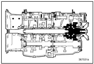
Figure 354 — Rear Mainshaft and Synchronizer Component Locator (T313L/T318L Shown)
