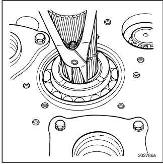
Figure 102 — Removing Rear Bearing Snap Ring
