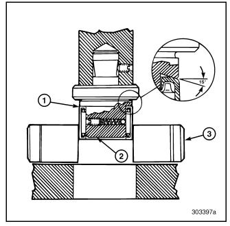
Figure 308 — Installation of Drawn Cup Bearings
