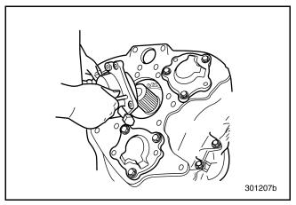
Figure 84 — Rear Mainshaft Bearing Cover Removed
