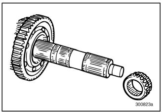
Figure 207 — Removing Lo/Reverse Sliding Clutch from Mainshaft (T313L/T318L Shown)
