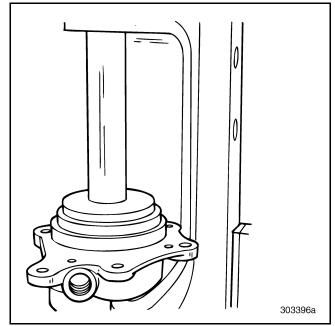
Figure 343 — Pressing Bearing into Cover
