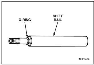
Figure 463 — Installing Shift Rail O-Ring
