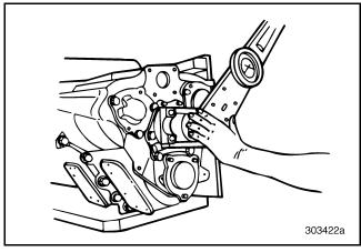
Figure 568 — Tightening Clamp Plate Capscrew (T313LR/T318LR Shown)
