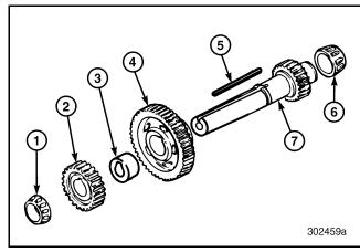
Figure 598 — Exploded View of Rear Countershaft
