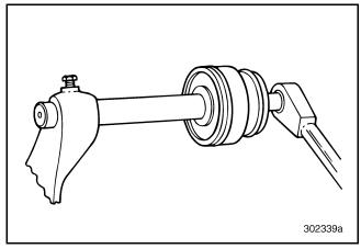
Figure 464 — Tightening Shift Piston Retaining Nut
