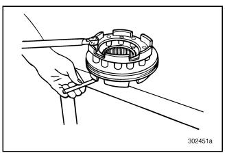
Figure 261 — Removing 12-Point Screws
