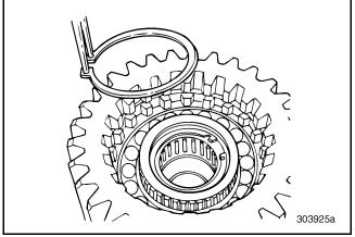
Figure 387 — Installing Shaft Snap Ring (T313L/T318L Shown)
