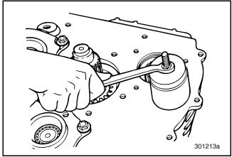
Figure 118 — Using Tool J 34630 to Remove Reverse Idler Shaft
