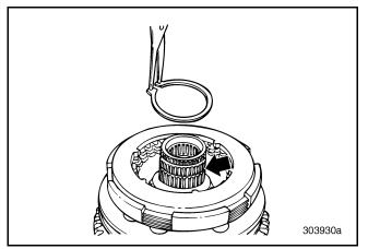
Figure 238 — Removing Shaft Snap Ring (T313L/T318L Shown)
