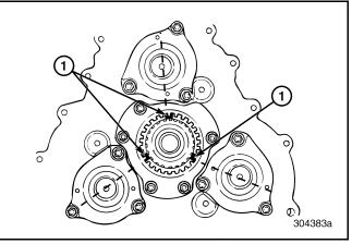
Figure 547 — Installing and Aligning Lo-Split Gear
