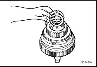
Figure 393 — Installing Thrust Washers (T313L21/T318L21 Shown)
