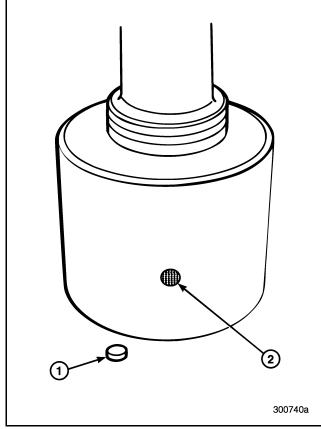
Figure 461 — Shift Cylinder Breather Vent
