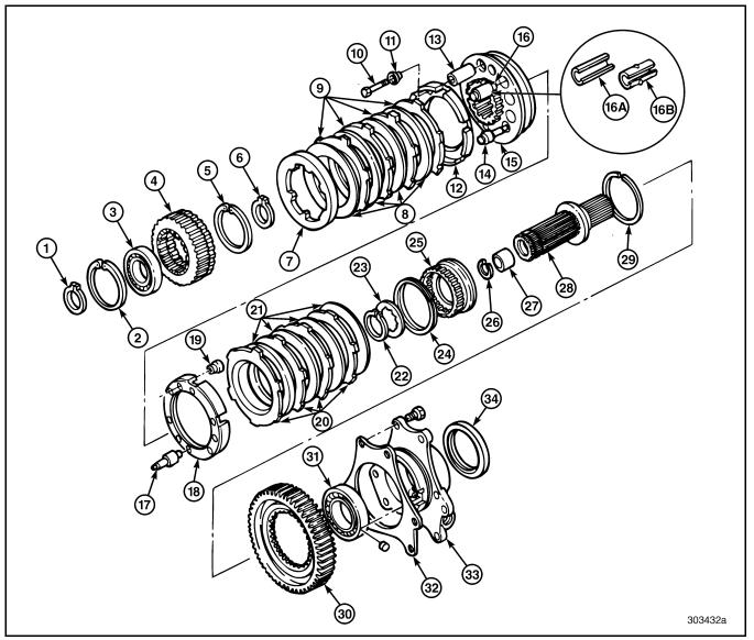
Figure 357 — Exploded View of: T313–T318(L)(LR) Rear Mainshaft and Synchronizer Assembly
