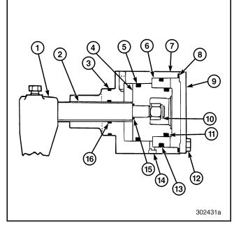
Figure 604 — Cutaway View of Three-Position Range Shift Cylinder
