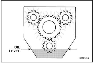
Figure 9 — Splash Lubrication
