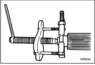
Figure 225 — Removing Front Spigot Bearing Inner Race
