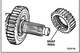
Figure 411 — Installing Fourth Speed Gear
