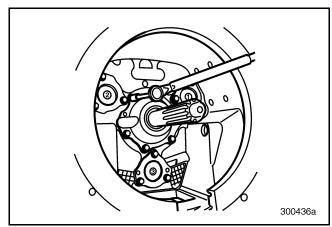
Figure 544 — Tightening Main Drive Pinion Bearing Cover Capscrews
