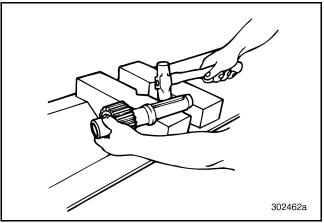
Figure 314 — Installing Key
