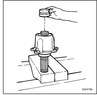
Figure 351 — Installing Spacer
