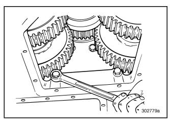
Figure 91 — Removing Outer Rear Case-to-Main Case Capscrews
