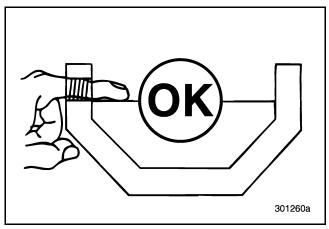
Figure 56 — Correct Oil Level
