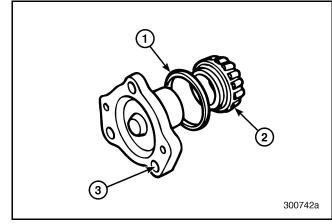
Figure 336 — Exploded View of Front Countershaft Front Bearing Cover
