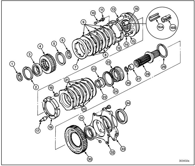
Figure 602 — Exploded View of Rear Mainshaft and Synchronizer Assembly, T313–T318(L)(LR)
