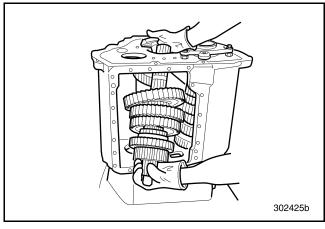
Figure 522 — Installing Mainshaft into Case
