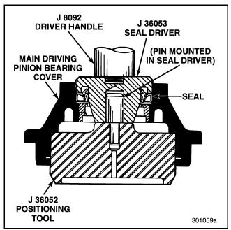
Figure 430 — Installing Bearing Cover Oil Seal
