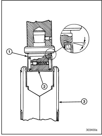
Figure 369 — Installation of Drawn Cup Bearings (T313L/T318L Shown)
