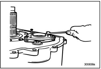
Figure 100 — Removing No. 2 Front Countershaft Rear Bearing Cover (T313L/T318L Shown)
