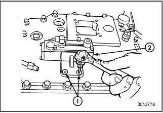
Figure 579 — Tightening Range Shift Interlock Valve Screws
