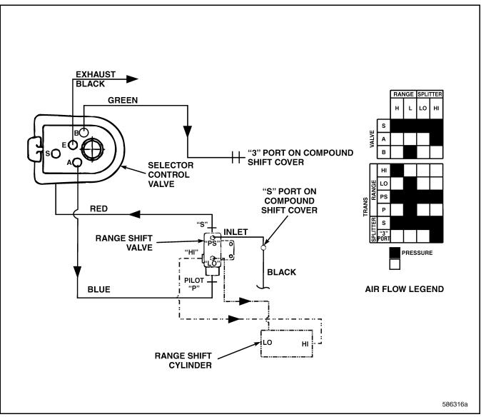
Figure 590 — Air Control Schematic
