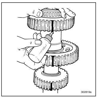
Figure 550 — Marking Rear Countershaft Gears
