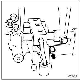
Figure 511 — Installing Nut and Washers
