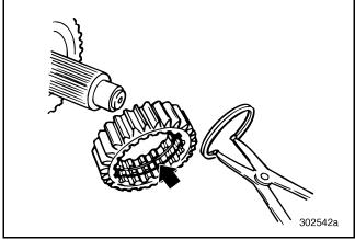
Figure 410 — Installing Snap Ring into Fourth Speed Gear
