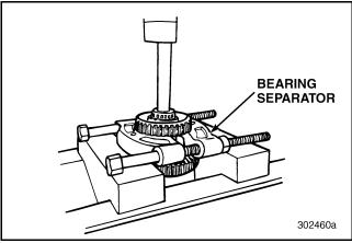
Figure 292 — Pressing off Lo-Split Gear and Bearing Cone
