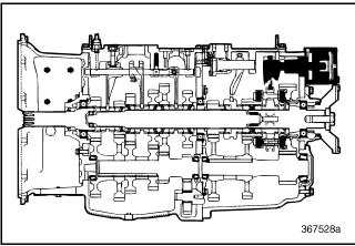
Figure 167 — Range Shift Cylinder Component Locator (T313L/T318L Shown)
