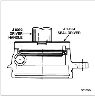
Figure 304 — Rear Mainshaft Bearing Cover Oil Seal Tools
