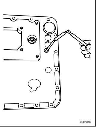
Figure 154 — Removing Reverse Light Switch Rod
