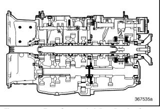
Figure 285 — Front Countershaft Rear Bearing Cover Component Locator (T313L/T318L Shown)
