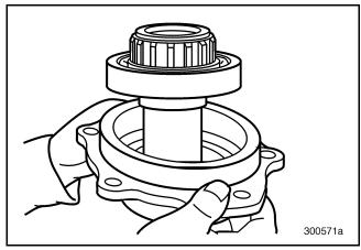
Figure 197 — Removing Main Drive Pinion Shaft and Bearing from Cover
