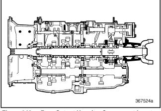
Figure 346 — Rear Output Housing Component Locator (T313L21/T318L21 Shown)
