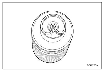
Figure 444 — Inserting Teflon<sup>®</sup> Seal in Nose of Insertion Tool (Tool No. J 47357)
