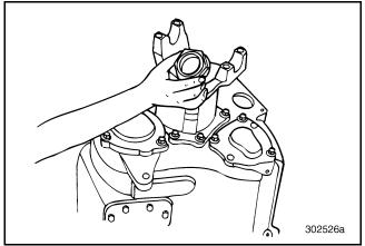
Figure 566 — Installing Drive Yoke and Nut (T313L21/T318L21 Shown)
