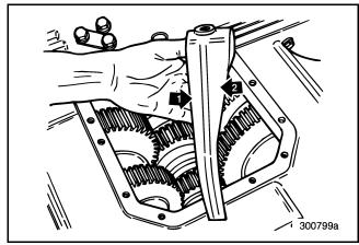
Figure 569 — Installing Range Shift Fork
