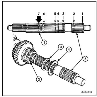
Figure 414 — Installing Internal- and External-Toothed Thrust Washers (T313L/T318L Shown)
