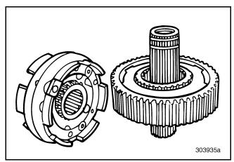
Figure 249 — Synchronizer Assembly Removed (T313L/T318L Shown)
