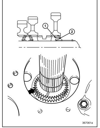
Figure 530 — Installing Internal-Toothed Thrust Washer
