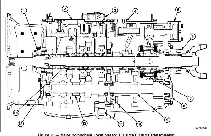
Figure 53 — Major Component Locations for T313L21/T318L21 Transmission
