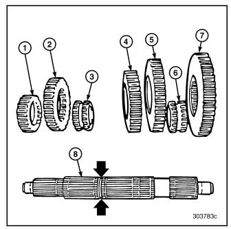
Figure 203 — View of Mainshaft and Gears (T313L/T318L Shown)
