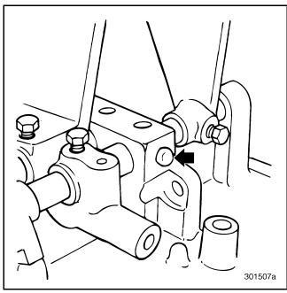
Figure 131 — Remove Interlock Ball from Cover
