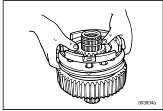
Figure 248 — Removing Synchronizer Assembly (T313L/T318L Shown)
