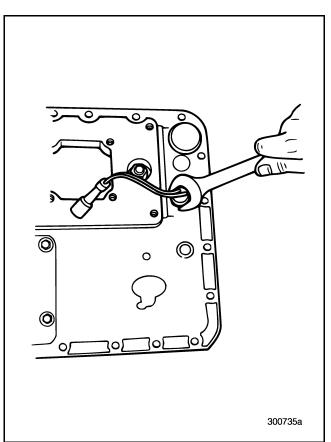
Figure 153 — Removing Reverse Light Switch
