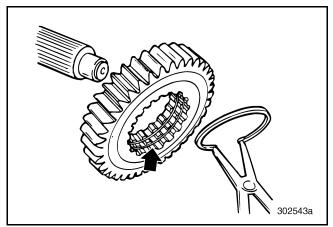
Figure 220 — Removing Second Speed Gear Snap Ring
