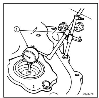
Figure 527 — Measuring Countershaft End Play
