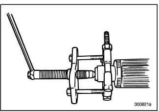
Figure 227 — Removing Rear Spigot Bearing Inner Race (T313L/T318L Shown)
