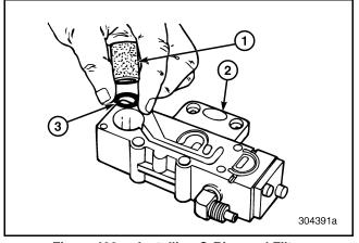
Figure 438 — Installing O-Ring and Filter
