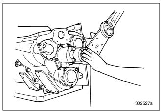
Figure 567 — Torquing Drive Yoke Nut (T313L21/T318L21 Shown)
