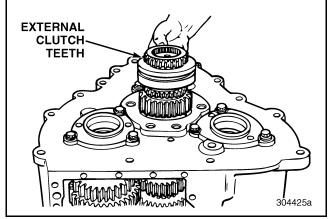
Figure 549 — Installing the Sliding Clutch
