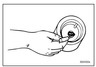
Figure 468 — Installing Shift Cylinder Inside O-Ring
