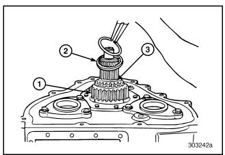
Figure 99 — Removing Snap Ring, Thrust Washer and Lo-Split Gear (T313L/T318L Shown)
