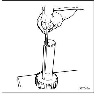
Figure 283 — Removing Key
