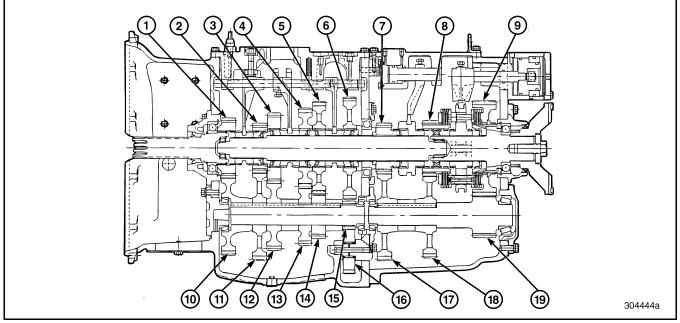
Figure 584 — Gear Identification (T313/T318 Shown)
