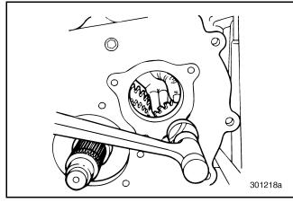
Figure 525 — Installing No. 2 Reverse Idler Shaft and Gear
