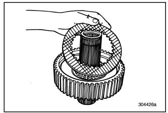
Figure 376 — Installing Friction Disc (T313L/T318L Shown)
