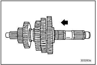
Figure 424 — Moving Sliding Clutch and Reverse Speed Gear Forward (T313L/T318L Shown)
