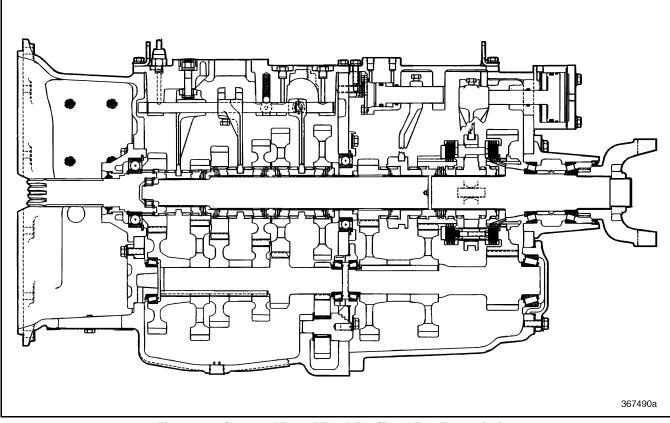
Figure 7 — Cutaway View of T313LR21/T318LR21 Transmission
