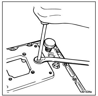
Figure 577 — Adjusting Eccentric Pin
