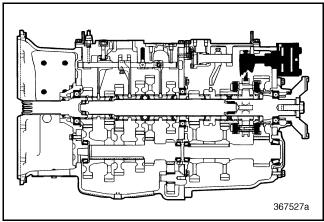
Figure 441 — Range Shift Cylinder Locator (T313L/T318L Shown)
