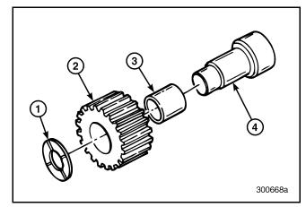
Figure 597 — Exploded View of Reverse Idler Gear Assembly
