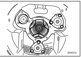
Figure 534 — Gear Timing Marks Aligned
