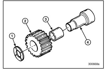
Figure 299 — Exploded View of Reverse Idler Gear Assembly
