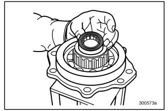
Figure 195 — Spigot Bearing Removed from Main Drive Pinion Shaft
