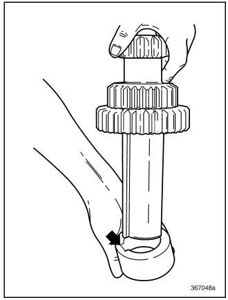
Figure 329 — Installing First and Second Gear Spacer
