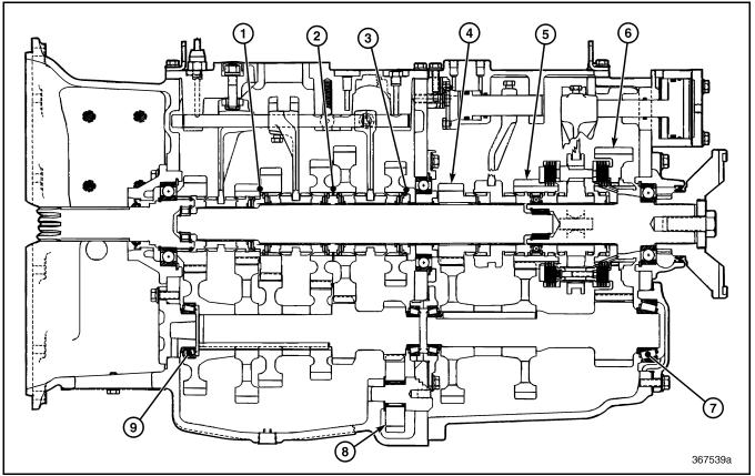
Figure 588 — Gear End Play and Bearing Preload (T313L/T318L Shown)
