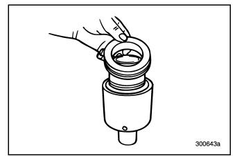
Figure 170 — Removing Sleeve from Piston
