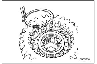
Figure 231 — Removing Smaller Mainshaft Snap Ring (T313L/T318L Shown)
