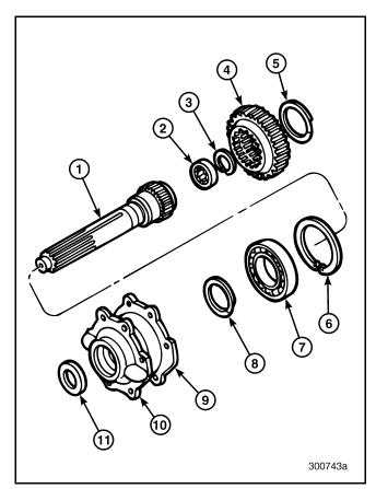
Figure 596 — Exploded View of Main Drive Pinion
