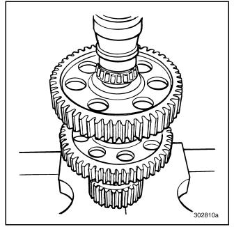
Figure 318 — Pressing on Front Bearing Cone
