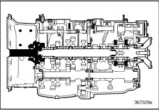
Figure 189 -Main Drive Pinion Component Locator (T313L/T318L Shown)
