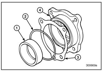
Figure 607 — Exploded View of Rear Countershaft Bearing Cover
