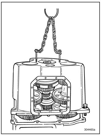
Figure 554 — Installing Rear Case
