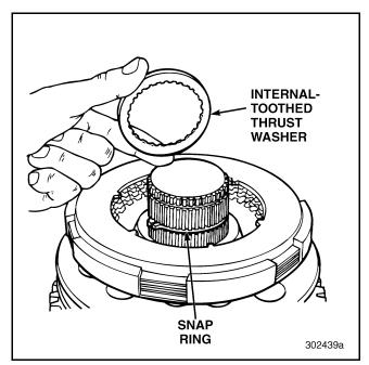
Figure 389 — Installing Internal-Toothed Thrust Washer (T313L21/T318L21 Shown)
