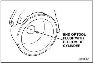
Figure 449 — Installer/Sizer Tool Fully Inserted and End Flush with Bottom of Cylinder
