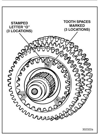
Figure 513 — Gear Tooth Spaces Marked for Timing
