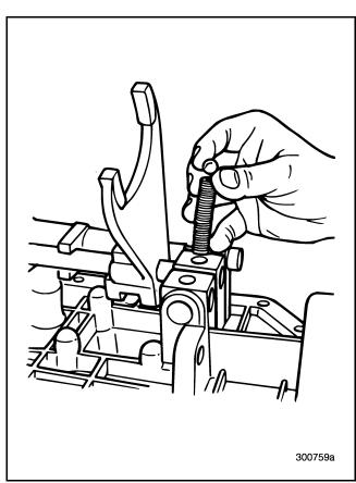
Figure 143 — Removing Poppet Ball and Spring
