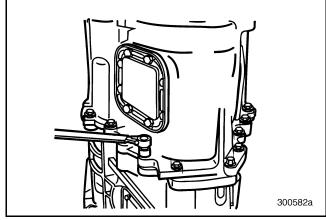
Figure 555 — Tightening Outer Case-to-Case Capscrews
