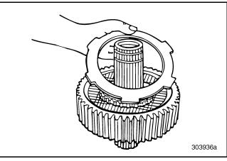
Figure 250 — Removing Reaction Disc (T313L/T318L Shown)
