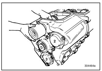
Figure 75 — Removing Range Shift Cylinder
