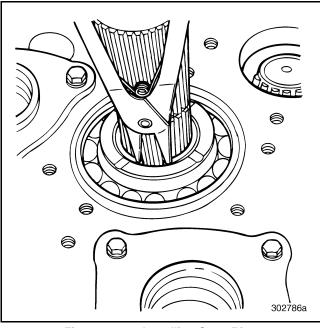
Figure 538 — Installing Snap Ring
