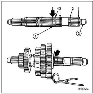
Figure 423 — Installing Reverse Speed Gear Snap Ring onto Mainshaft (T313L/T318L Shown)
