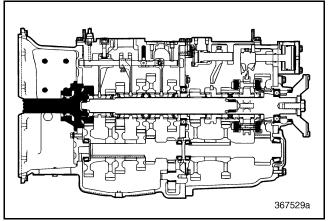
Figure 425 — Main Drive Pinion Component Locator (T313L/T318L Shown)
