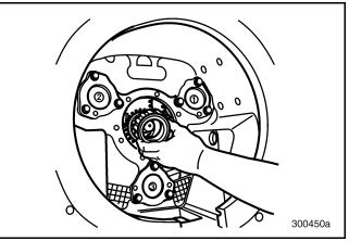
Figure 113 — Removing Sliding Clutch
