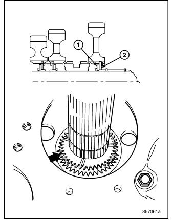
Figure 107 — Removing External- and Internal-Toothed Thrust Washers
