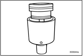
Figure 169 — Piston Assembly Partially Removed
