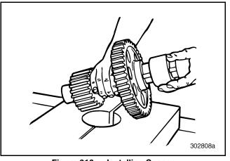
Figure 316 — Installing Spacer
