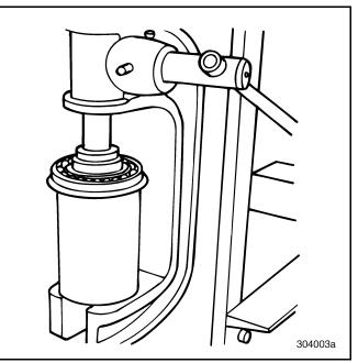
Figure 104 — Pressing Sleeve Out of Bearing
