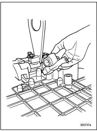
Figure 500 — Installing Lo/Reverse Shifter
