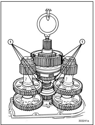
Figure 552 — Installing Rear Mainshaft and Synchronizer Assembly (T313LR/T318LR Shown)
