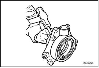
Figure 269 — Using Hammer and Blunt Punch to Remove Oil Seal
