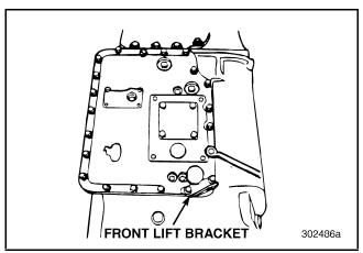
Figure 576 — Tightening Main Case Shift Cover Capscrews
