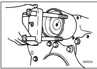
Figure 73 — Removing Range Shift Cylinder Cover
