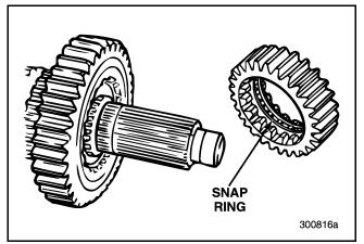
Figure 217 — Removing Fourth Speed Gear
