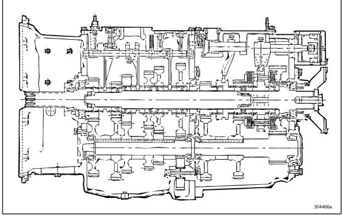
Figure 3 — Cutaway View of T313/T318 Transmission
