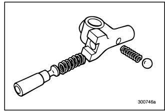
Figure 152 — Lo/Reverse Shifter Disassembled
