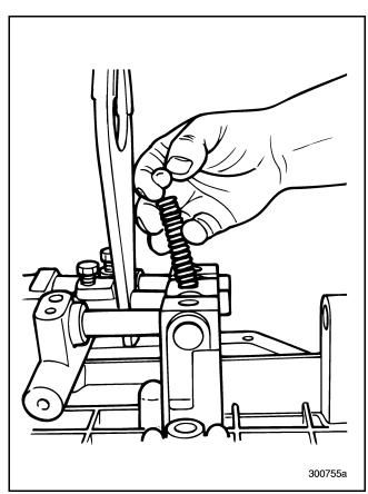
Figure 137 — Removing Poppet Ball and Spring
