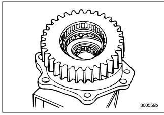
Figure 193 — Removing Main Drive Pinion Gear
