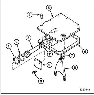
Figure 160 — Exploded View of Rear Case Shift Cover
