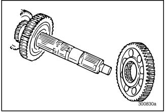
Figure 210 — Removing Lo-Speed Gear (T313L/T318L Shown)
