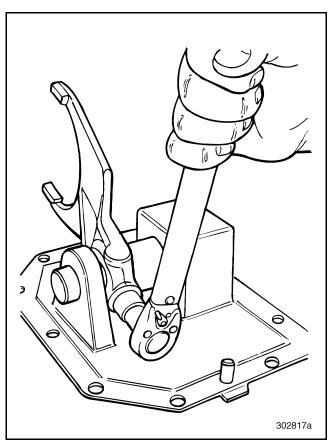
Figure 477 — Tightening Shift Fork Setscrew
