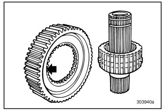
Figure 372 — Installing Lo-Range Gear
