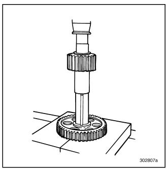
Figure 315 — Pressing on Hi-Range/Hi-Split Gear
