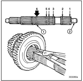
Figure 420 — Installing Internal- and External-Toothed Thrust Washers (T313L/T318L Shown)
