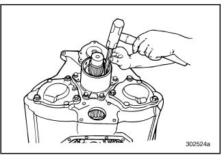
Figure 564 — Seating the Bearing Cone and Spacer (T313L21/T318L21 Shown)
