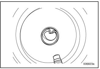
Figure 447 — Seal Properly Installed in Shift Rail Bore
