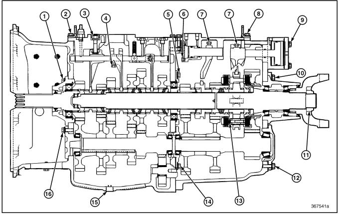
Figure 583 — Torque Specifications (T313L21/T318L21 Shown)
