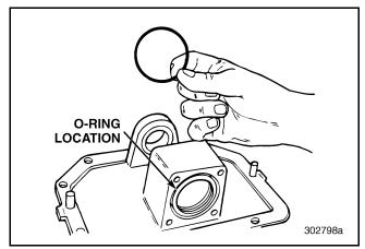
Figure 164 — Removing Piston Cover O-Ring
