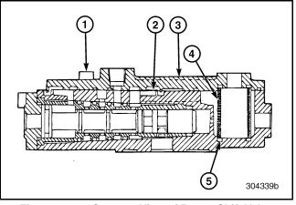
Figure 186 — Cutaway View of Range Shift Valve Assembly
