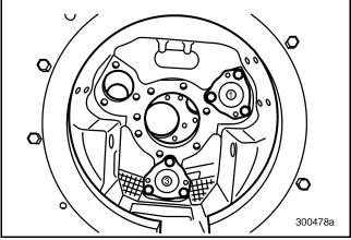
Figure 514 — No. 1 and No. 3 Front Countershaft Front Bearing Covers Installed
