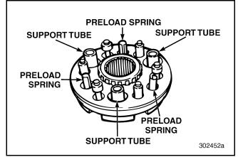
Figure 262 — Remove Synchronizer Support Tubes and **Preload Springs**
