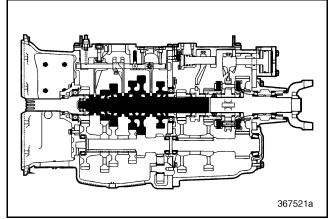
Figure 397 — Front Mainshaft Component Locator (T313L21/T318L21 Shown)
