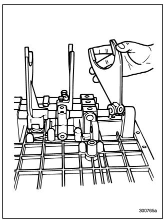
Figure 504 — Installing Lo/Reverse Shift Fork
