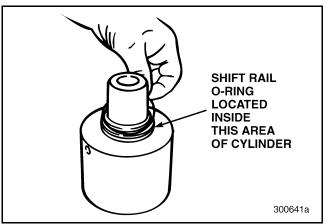
Figure 467 — Installing Shift Cylinder Outside O-Ring
