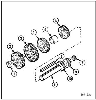
Figure 278 — Exploded View of Front Countershaft
