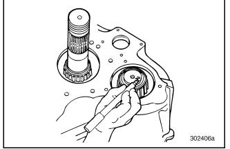
Figure 90 — Marking Rear Countershafts (T313L21/T318L21 Shown)
