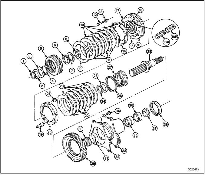
Figure 603 — Exploded View of Rear Output Shaft and Synchronizer Assembly, T313–T318(21)(L21)(LR21)
