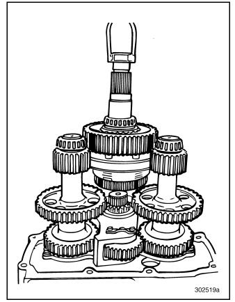
Figure 553 — Installing Output Shaft and Synchronizer Assembly (T313LR21/T318LR21 Shown)
