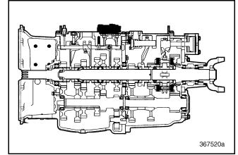
Figure 436 — Range Shift Valve Component Locator (T313L21/T318L21 Shown)
