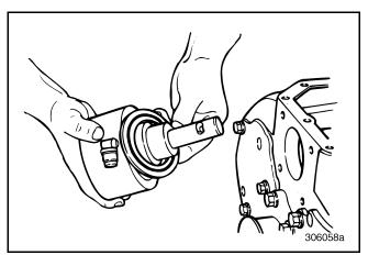
Figure 76 — Two-Position Shift Cylinder Gasket
