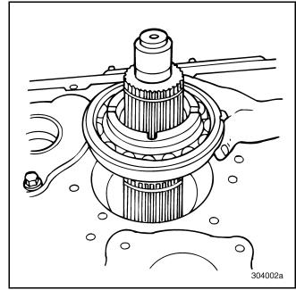
Figure 537 — Installing Front Mainshaft Rear Bearing (T313LR/T318LR Shown)
