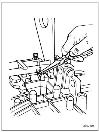
Figure 145 — Removing Interlock Pin
