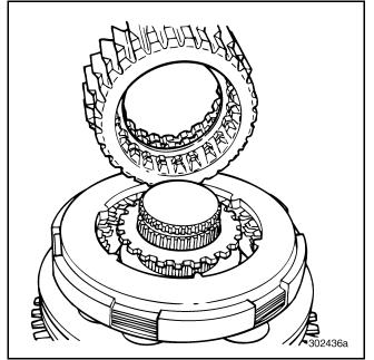
Figure 241 — Removing Hi-Range/Hi-Split Gear (T313L21/T318L21 Shown)
