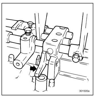
Figure 510 — Installing Interlock Rocker and Bolt
