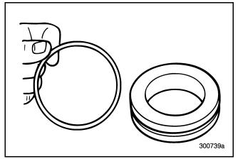
Figure 177 — Removing O-Ring from Sleeve
