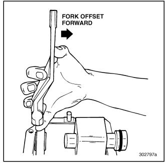
Figure 163 — Removing Piston and Shift Fork
