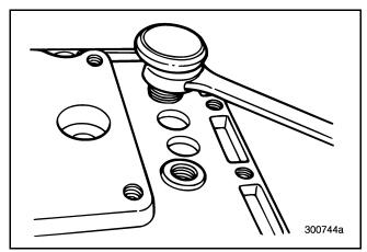
Figure 158 — Removing Breather Vent
