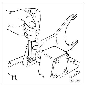
Figure 161 — Removing Setscrew
