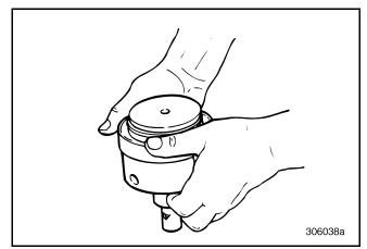
Figure 181 — Piston Assembly Partially Removed
