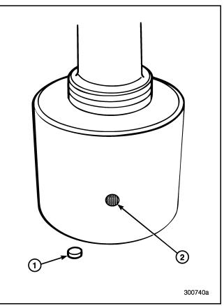
Figure 178 — Shift Cylinder Breather Vent Shown Removed (1) and Installed (2)
