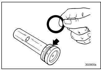
Figure 473 — Installing Shift Piston O-Ring
