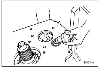
Figure 119 — Removing Reverse Idler Gear and Shaft
