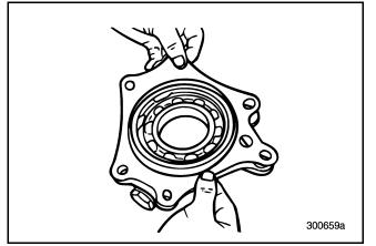
Figure 345 — Installing Gasket onto Cover
