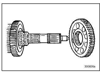
Figure 422 — Installing Reverse Speed Gear onto Mainshaft (T313L/T318L Shown)
