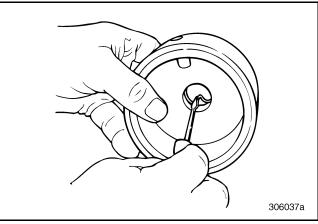
Figure 182 — Removing Teflon<sup>®</sup> Seal and O-Ring Expander
