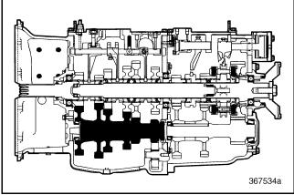
Figure 277 — Front Countershaft Component Locator (T313L/T318L Shown)
