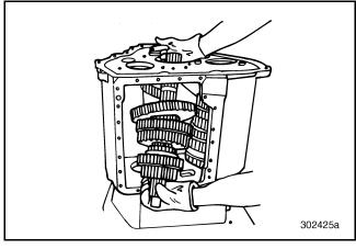
Figure 122 — Removing the Mainshaft
