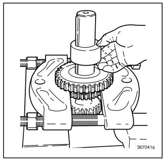
Figure 280 — Removing First/Second Gear Spacer
