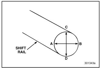
Figure 302 — Measuring Shift Rail
