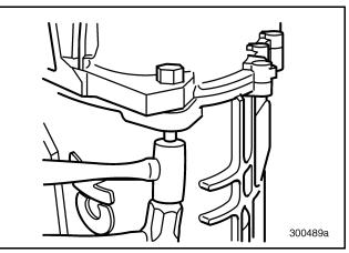
Figure 93 — Removing Dowel Bolts
