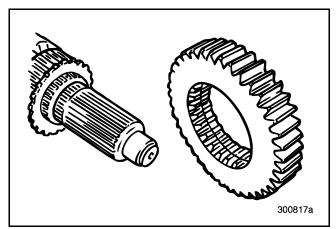
Figure 219 — Removing Second Speed Gear
