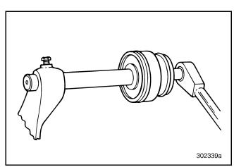
Figure 175 — Removing Shift Piston Retaining Nut
