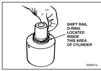
Figure 171 — Removing Shift Cylinder Outside O-Ring
