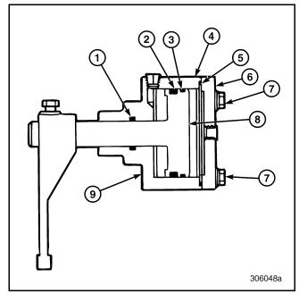
Figure 442 — Cutaway View of Range Shift Cylinder
