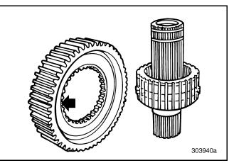
Figure 255 — Removing Lo-Range Gear from Hub (T313L/T318L Shown)
