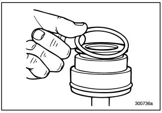
Figure 466 — Installing Shift Piston Rear O-Ring
