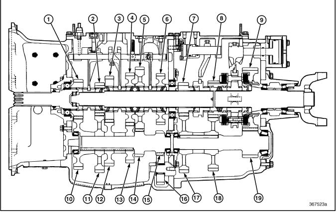
Figure 586 — Gear Identification (T313L21/T318L21 Shown)
