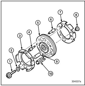
Figure 356 — Exploded View of Synchronizer
