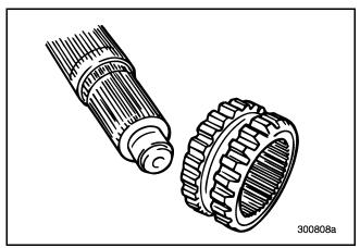
Figure 223 — Removing First/Second Sliding Clutch
