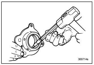
Figure 288 — Removing Rear Bearing Cup
