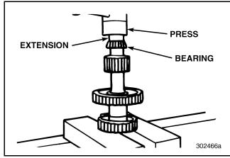
Figure 319 — Pressing on Rear Bearing Cone
