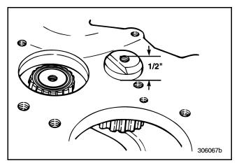
Figure 520 — Reverse Idler Shaft Protrusion
