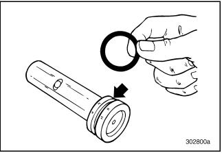
Figure 166 — Removing Piston O-Ring
