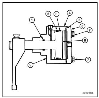
Figure 180 — Range Shift Cylinder Cutaway View
