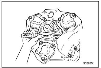
Figure 82 — Removing Rear Mainshaft Bearing Cover Capscrews
