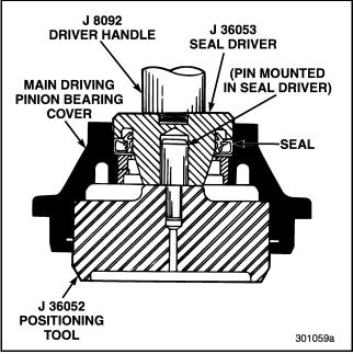
Figure 303 — Main Drive Pinion Oil Seal Tools
