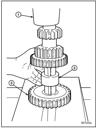
Figure 331 — Pressing Second Speed Gear onto Shaft
