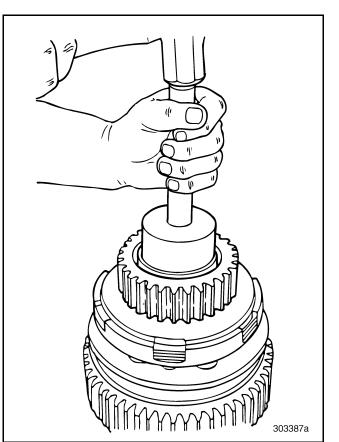
Figure 386 — Installing Ball Bearing (T313L/T318L Shown)
