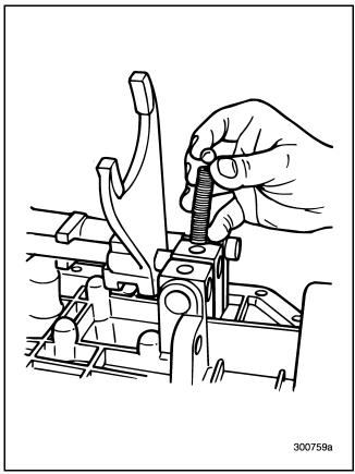
Figure 495 — Installing Poppet Ball and Spring
