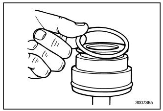
Figure 173 — Removing O-Ring from Rear of Piston
