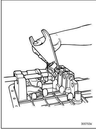
Figure 146 — Removing First/Second Shift Fork
