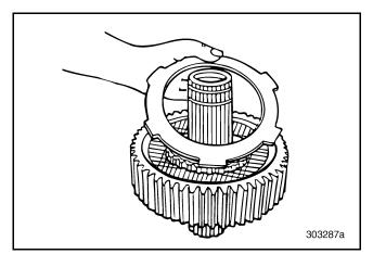
Figure 377 — Installing Reaction Disc (T313L/T318L Shown)
