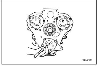
Figure 86 — Mark Rear Countershaft Bearing Covers for Placement
