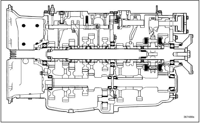
Figure 4 — Cutaway View of T313L/T318L Transmission
