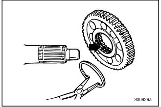
Figure 417 — Installing Snap Ring into Lo-Speed Gear (T313L/T318L Shown)
