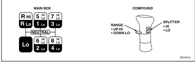
Figure 12 — T313(L)(LR)(21)(L21)(LR21) Shift Pattern
