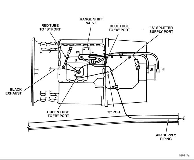
Figure 591 — Air Piping Diagram
