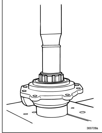
Figure 431 — Installing Main Drive Pinion Assembly into Drive Pinion Bearing Cover
