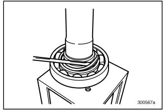
Figure 198 — Removing Spiral Snap Ring from Main Drive Pinion
