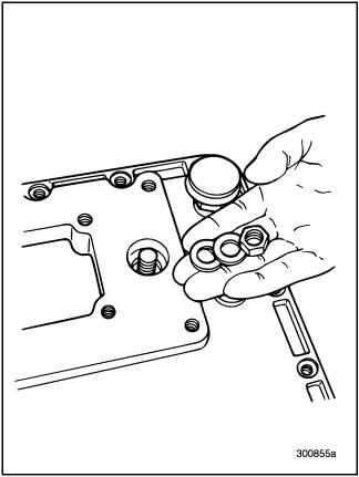
Figure 483 — Installing Washers and Nut
