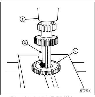
Figure 328 — Installing First (Fifth) Gear on Countershaft
