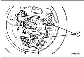
Figure 111 — Oil Pump Discharge Line (if Equipped)
