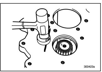
Figure 519 — Tapping Reverse Idler Shaft into Place
