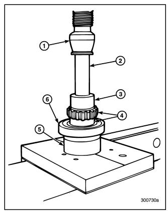
Figure 427 — Installing Main Drive Pinion Bearing
