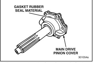
Figure 541 — Installing Cover Gasket with Sealing Material Facing Cover
