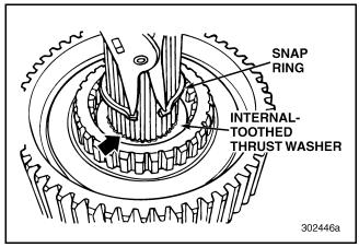
Figure 375 — Installing Lo-Range Gear Hub Shaft Snap Ring
