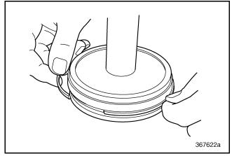
Figure 452 — Installing Wiper Ring in Upper (Thin) Piston Groove
