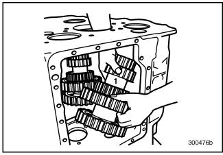
Figure 123 — Removing No. 1 Upper Left Countershaft
