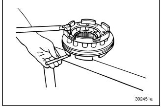
Figure 366 — Tightening 12-Point Screws
