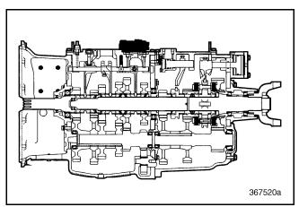
Figure 185 — Range Shift Valve Component Locator (T313L21/T318L21 Shown)
