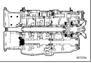
Figure 273 — Front Countershaft Front Bearing Cover Component Locator (T313L/T318L Shown)
