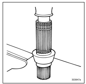
Figure 368 — Installing Spigot Bearing (T313L/T318L Shown)
