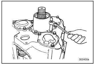
Figure 79 — Removing Extended Output Housing Capscrews (T313L21/T318L21 Shown)
