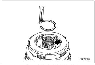
Figure 382 — Installing Shaft Snap Ring (T313L/T318L Shown)
