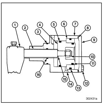
Figure 460 — Cutaway View of Range Shift Cylinder
