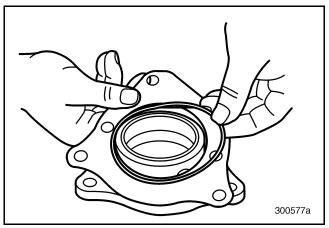
Figure 296 — Removing Cover Shims and O-Ring
