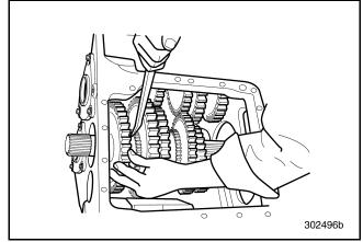
Figure 526 — Sliding Lo/Reverse Sliding Clutch and Reverse Speed Gear to Engage Gear Teeth (T313L21/T318L21 Shown)
