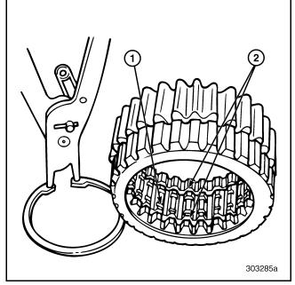
Figure 383 — Installing Gear Snap Ring (T313L/T318L Shown)
