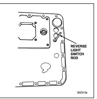
Figure 485 — Installing Reverse Light Switch Rod
