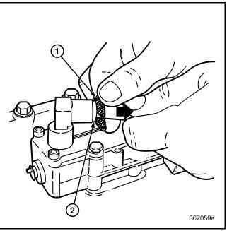
Figure 61 — Removing Air Lines
