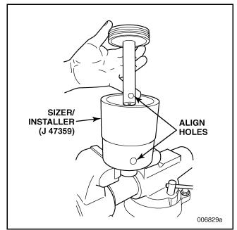
Figure 457 — Aligning Shift Fork Locking Bolt Hole with Air Fitting Port in Cylinder Housing
