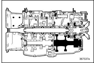
Figure 312 — Rear Countershaft Component Locator (T313L/T318L Shown)
