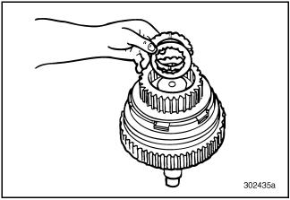
Figure 240 — Removing Thrust Washers (T313L21/T318L21 Shown)
