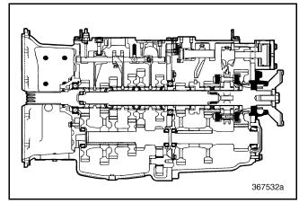
Figure 339 — Rear Mainshaft Bearing Cover Component Locator (T313L/T318L Shown)
