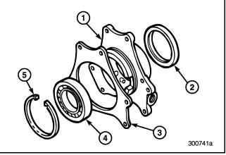
Figure 340 — Exploded View of Rear Mainshaft Bearing Cover
