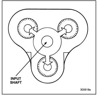
Figure 8 — Equal Torque Distribution
