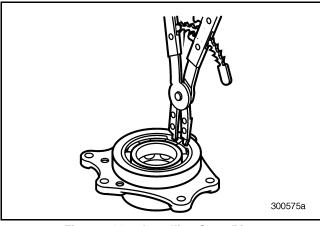
Figure 344 — Installing Snap Ring
