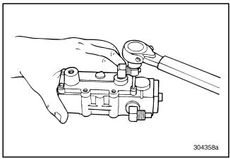
Figure 440 — Installing Top Cover
