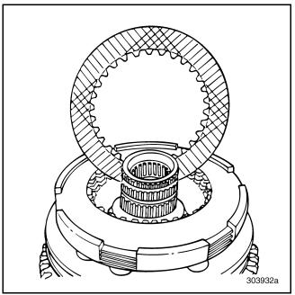
Figure 246 — Removing Friction Disc (T313L/T318L Shown)
