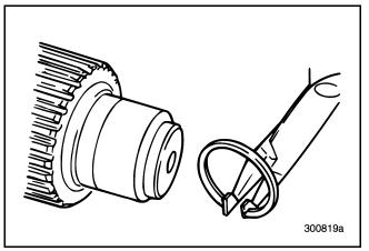
Figure 401 — Installing Inner Race Snap Ring
