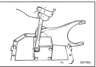
Figure 162 — Removing Cover Capscrews
