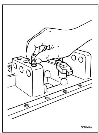
Figure 151 — Removing Poppet Ball and Spring
