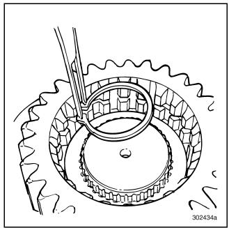
Figure 239 — Removing Snap Ring from Front of Shaft (T313L21/T318L21 Shown)
