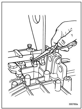
Figure 493 — Installing Pin into First/Second Shift Rail
