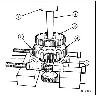
Figure 279 — Pressing Gears off Shaft
