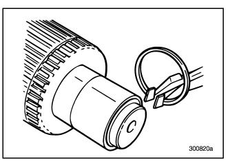
Figure 403 — Installing Inner Race Snap Ring (T313L/T318L Shown)
