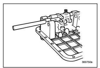
Figure 491 — Installing First/Second Shift Rail
