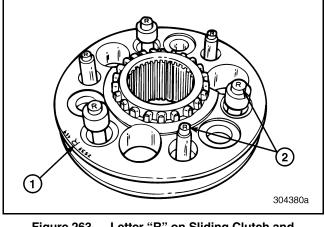
Figure 263 — Letter "R" on Sliding Clutch and Synchronizer Pins
