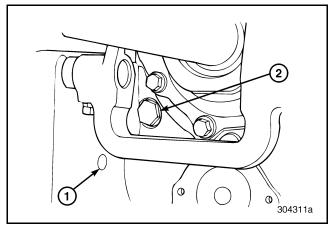
Figure 10 — Transmission Case Oil Cooler Line Plugs
