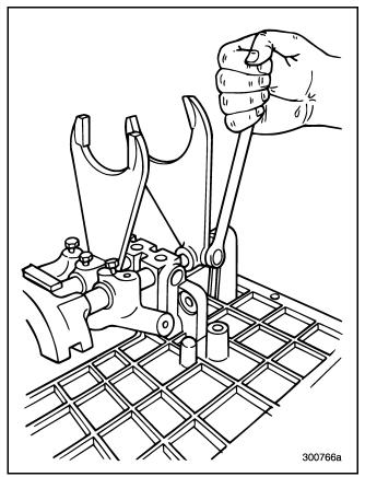
Figure 132 — Removing Setscrew from Lo/Reverse Shift Fork
