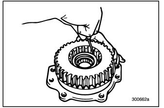
Figure 434 — Installing Main Drive Pinion Gear and Spiral Snap Ring
