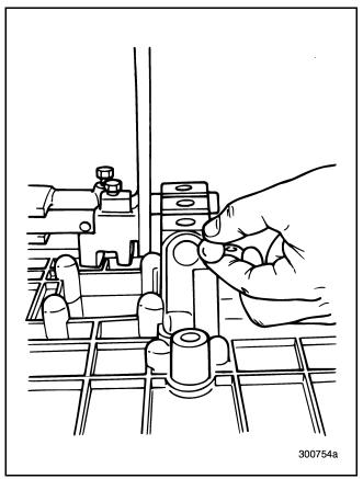
Figure 144 — Removing Interlock Ball
