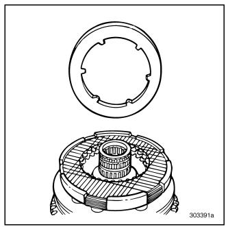
Figure 381 — Installing Spacer (T313L/T318L Shown)
