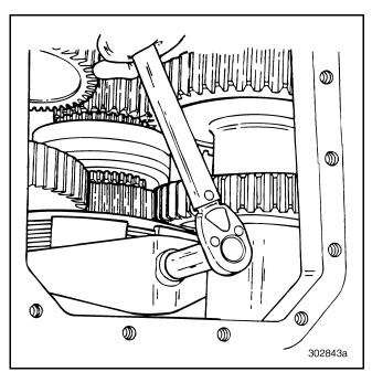
Figure 573 — Tightening Shift Fork Setscrew
