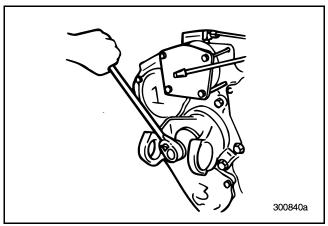
Figure 69 — Removing Clamp Plate and Capscrew (T313L/T318L Shown)
