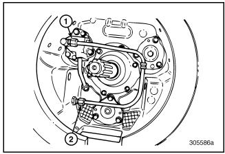
Figure 545 — Tighten Upper and Lower Discharge Tube Fittings
