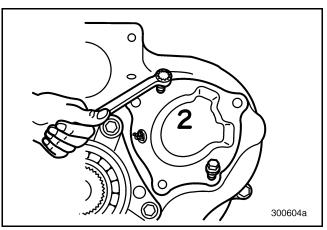
Figure 89 — Removing Bearing Cover
