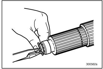
Figure 224 — Removing Front Spigot Bearing Inner Race Snap Ring
