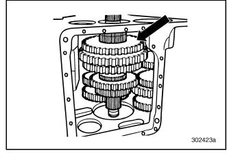
Figure 120 — Sliding Reverse Gear and Lo/Reverse Clutch Forward
