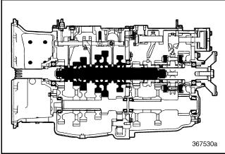
Figure 201 — Front Mainshaft Component Locator (T313L/T318L Shown)
