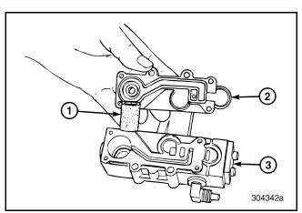
Figure 188 — Removing Sintered Bronze Filter
