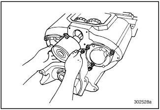
Figure 570 — Installing Range Shift Cylinder
