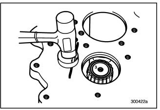
Figure 524 — Tapping Reverse Idler Shaft into Place
