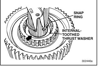
Figure 252 — Removing Shaft Snap Ring
