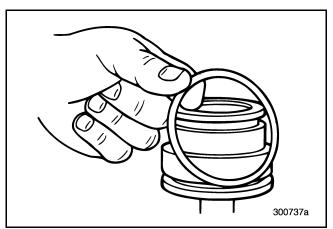
Figure 174 — Removing O-Ring from Front of Piston
