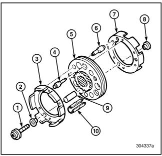
Figure 260 — Exploded View of Synchronizer
