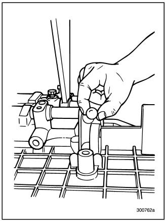
Figure 138 — Removing Interlock Ball
