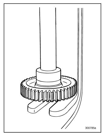
Figure 326 — Pressing Bearing Cup into Main Drive Gear
