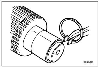
Figure 226 — Removing Rear Spigot Bearing Inner Race Snap Ring (T313L/T318L Shown)
