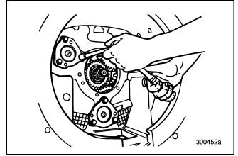
Figure 115 — Removing No. 2 Front Countershaft Front Bearing Cover Capscrews
