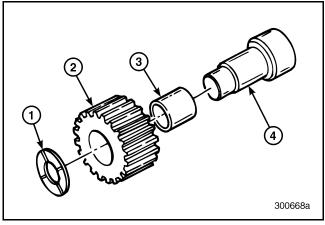
Figure 306 — Exploded View of Reverse Idler Gear Assembly
