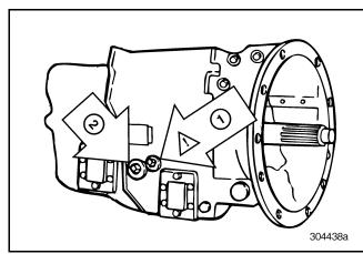
Figure 59 — Oil Filler and Check Plug
