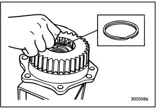
Figure 192 — Removing Snap Ring from Main Drive Pinion
