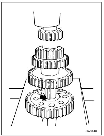
Figure 332 — Installing Fourth (Eighth) Speed Gear
