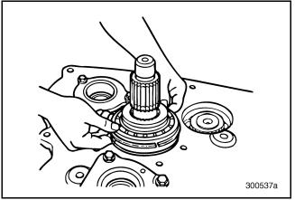
Figure 103 — Removing Front Mainshaft Rear Bearing (T313L/T318L Shown)
