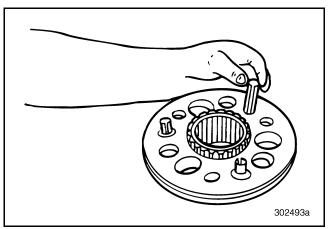
Figure 362 — Installing Preload Springs into Sliding Clutch
