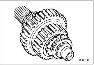
Figure 412 — Installing Internal- and External-Toothed Thrust Washers
