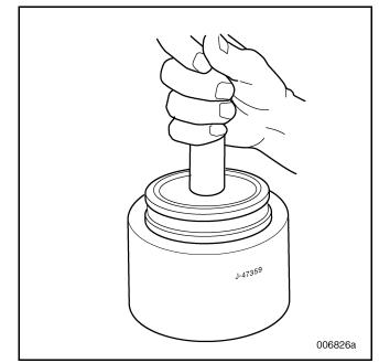
Figure 454 — Inserting Range Shift Piston into Seal Sizer/Piston Installer (Tool No. J 47359)
