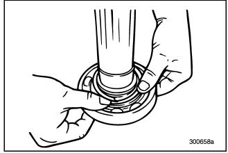
Figure 428 — Installing Spiral Snap Ring
