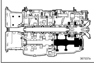
Figure 289 — Rear Countershaft Locator (T313L/T318L Shown)
