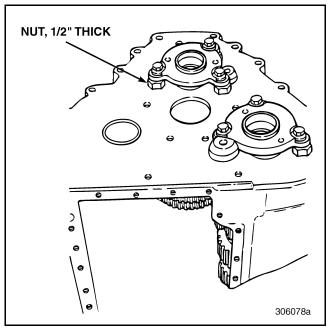
Figure 521 — Bearing Covers Temporarily Installed with Spacers
