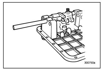
Figure 147 — Removing First/Second Shift Rail
