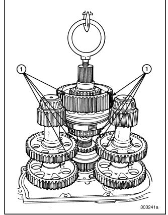
Figure 96 — Removing Mainshaft and Synchronizer Assembly (T313L/T318L Shown)
