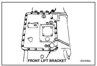
Figure 65 — Removing Main Case Shift Cover Capscrews
