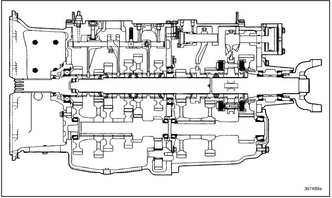
Figure 6 — Cutaway View of T313L21/T318L21 Transmission
