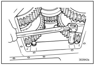
Figure 556 — Tightening Inner Case-to-Case Capscrews
