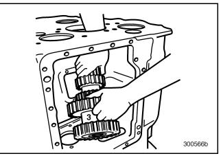
Figure 124 — Removing No. 3 Lower Countershaft
