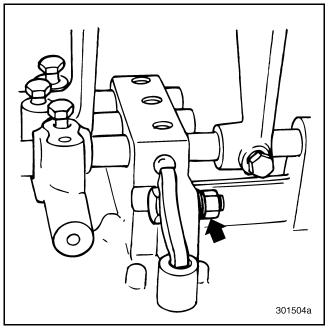
Figure 129 — Remove Nut and Washers
