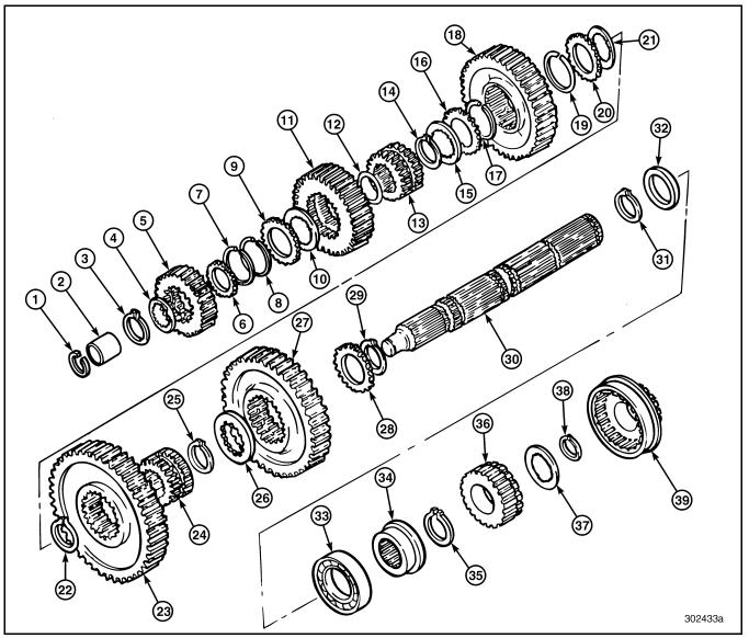
Figure 601 — Exploded View of Front Mainshaft, T313-T318(21)(L21)(LR21)
