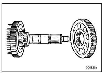
Figure 206 — Removing Reverse Gear from Mainshaft (T313L/T318L Shown)
