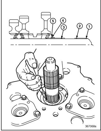
Figure 532 — Installing Spacer Snap Ring onto Mainshaft (T313L/T318L Shown)
