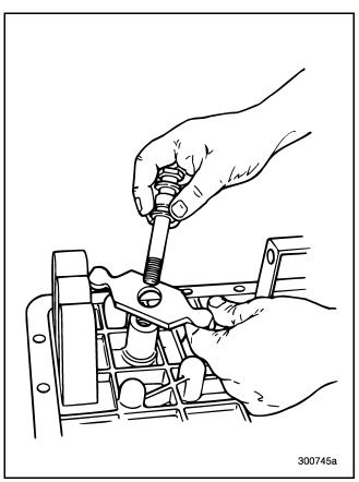
Figure 481 — Installing Third/Fourth Rocker Pin and Rocker Arm
