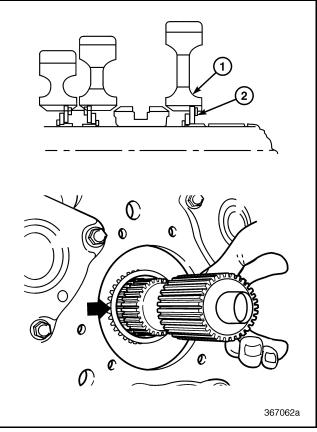
Figure 106 — Removing Snap Ring from Inside Reverse Speed Gear (T313L/T318L Shown)
