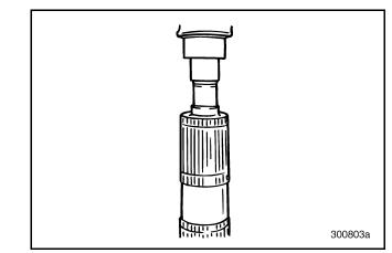
Figure 402 — Installing Spigot Bearing Inner Race (T313L/T318L Shown)
