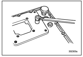
Figure 484 — Tightening Nut
