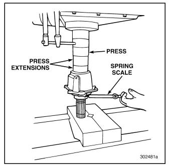
Figure 353 — Setup for Bearing Preload Adjustment Using Collapsible Spacer
