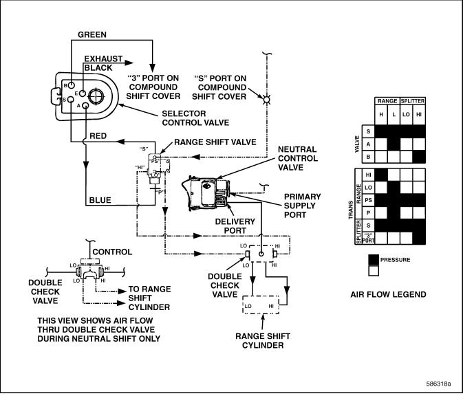
Figure 592 — Air Control Schematic
