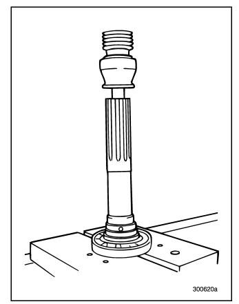
Figure 199 — Pressing Bearing Off Main Drive Pinion Shaft
