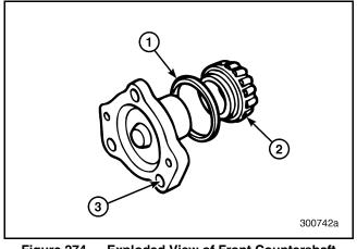
Figure 274 — Exploded View of Front Countershaft Front Bearing Cover
