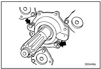
Figure 110 — Use Jackscrews to Remove Main Drive Pinion Assembly
