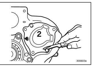
Figure 88 — Removing Jackscrew Plugs
