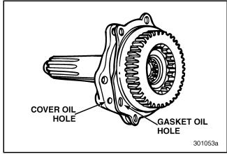
Figure 542 — Aligning Cover and Gasket Oil Holes
