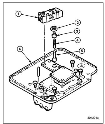
Figure 63 — Removing Range Shift Valve
