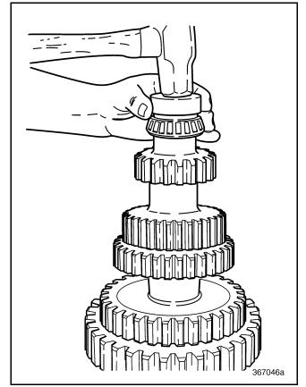
Figure 334 — Installing Rear Bearing Cone onto Shaft
