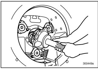
Figure 112 — Removing Main Drive Pinion Assembly
