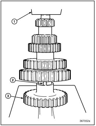
Figure 333 — Pressing Main Drive Gear onto Shaft
