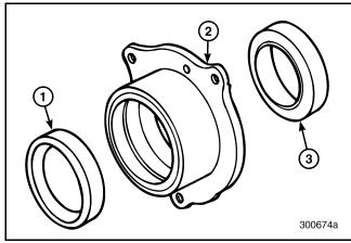
Figure 286 — Exploded View of Front Countershaft Rear Bearing Cover
