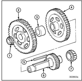
Figure 313 — Exploded View of Rear Countershaft
