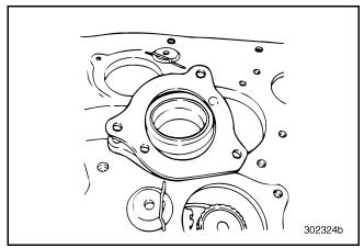
Figure 528 — Installing Shim Pack
