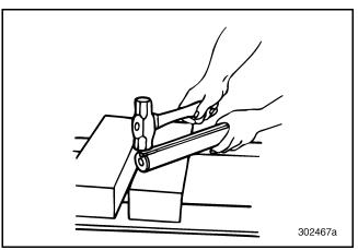
Figure 327 — Installing Key
