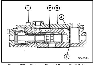
Figure 437 — Cutaway View of Range Shift Valve Assembly
