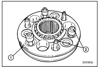
Figure 363 — Synchronizer Pins and Sliding Clutch Showing "R" Marks (Preload Springs Removed for Clarity)
