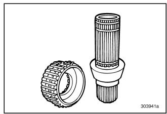
Figure 256 — Removing Lo-Range Gear Hub from Rear Mainshaft (T313L/T318L Shown)
