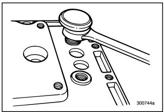
Figure 480 — Installing Breather Vent
