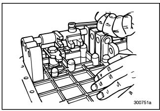
Figure 148 — Removing Setscrew from Third/Fourth Shifter
