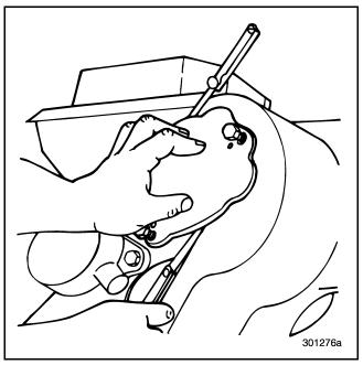
Figure 558 — Measuring with Standard Feeler Gauges
