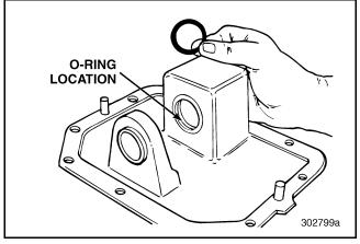
Figure 474 — Installing O-Ring into Rear of Housing
