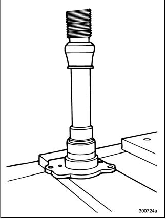
Figure 322 — Pressing Front Bearing Cup into Cover
