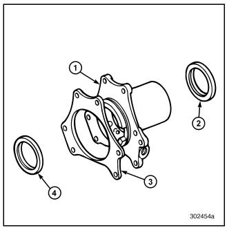
Figure 271 — Exploded View of Rear Output Housing
