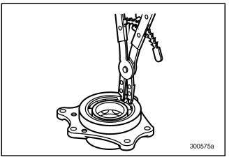
Figure 267 — Removing Snap Ring from Rear Mainshaft Bearing Cover
