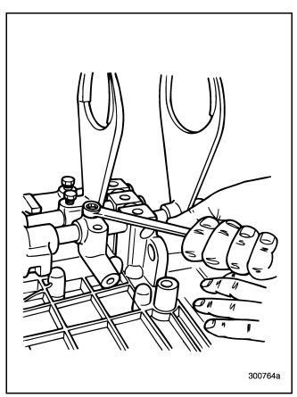
Figure 133 — Removing Setscrew from Lo/Reverse Shifter
