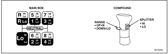
Figure 13 — T318(L)(LR)(21)(L21)(LR21) Shift Pattern
