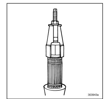
Figure 259 — Removing Spigot Bearing from Rear Mainshaft (T313L/T318L Shown)
