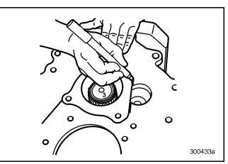
Figure 516 — Marking Idler Shaft Opening
