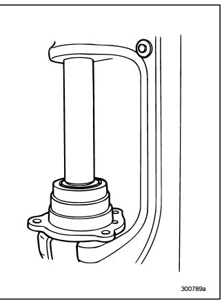
Figure 311 — Pressing Bearing Cup into Cover
