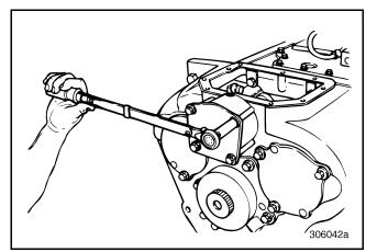
Figure 72 — Removing Range Shift Cylinder Capscrews
