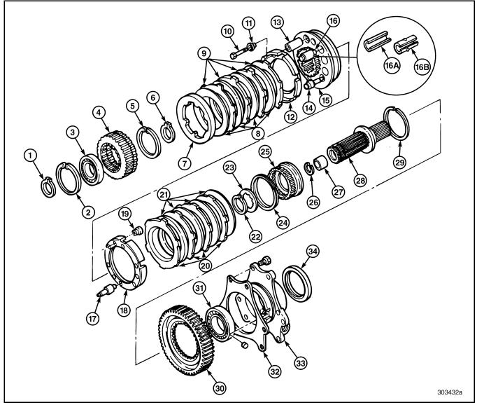
Figure 233 — Exploded View of: T313–T318(L)(LR) Rear Mainshaft and Synchronizer Assembly
