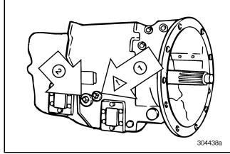
Figure 55 — Oil Filler and Check Plug
