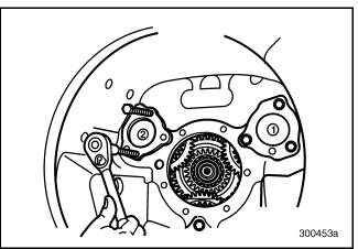
Figure 116 — Removing No. 2 Front Countershaft Front Bearing Cover
