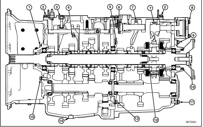
Figure 582 — Torque Specifications (T313L/T318L Shown)
