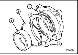
Figure 310 — Exploded View of Rear Countershaft Bearing Cover
