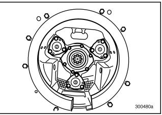
Figure 85 — Mark Front Countershaft Front Bearing Covers for Placement
