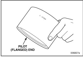
Figure 453 — Piston Assembled in Seal Sizer/Piston Installer (Tool No. J 47359)
