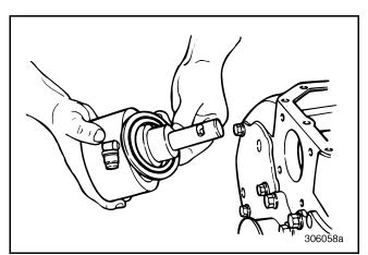
Figure 571 — Installing Shift Cylinder Gasket
