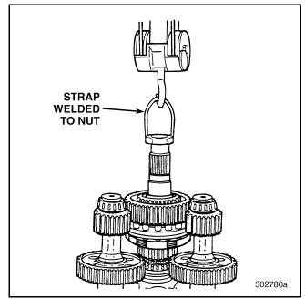
Figure 95 — Removing Mainshaft and Synchronizer Assembly (T313L21/T318L21 Shown)
