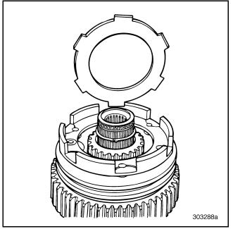
Figure 379 — Installing Reaction Disc (T313L/T318L Shown)
