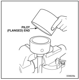
Figure 456 — Placing Seal Sizer/Piston Installer (Tool No. J 47359) on Cylinder Housing
