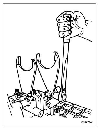
Figure 508 — Tightening Setscrew
