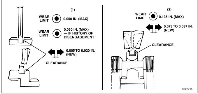
Figure 587 — Sliding Clutch Clearances
