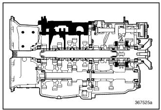
Figure 126 — Main Case Shift Cover Component Locator (T313L/T318L Shown)
