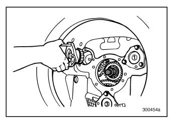
Figure 117 — No. 2 Front Countershaft Front Bearing Cover Removed
