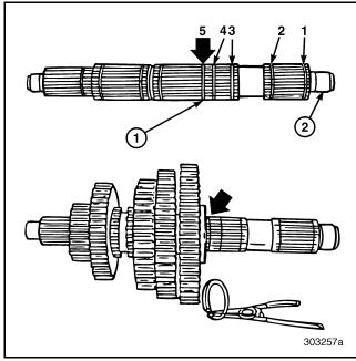
Figure 205 — Removing Reverse Gear Snap Ring (T313L/T318L Shown)
