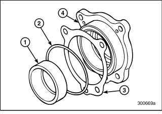
Figure 295 — Exploded View of Rear Countershaft Bearing Cover
