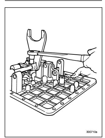
Figure 497 — Tightening Setscrew
