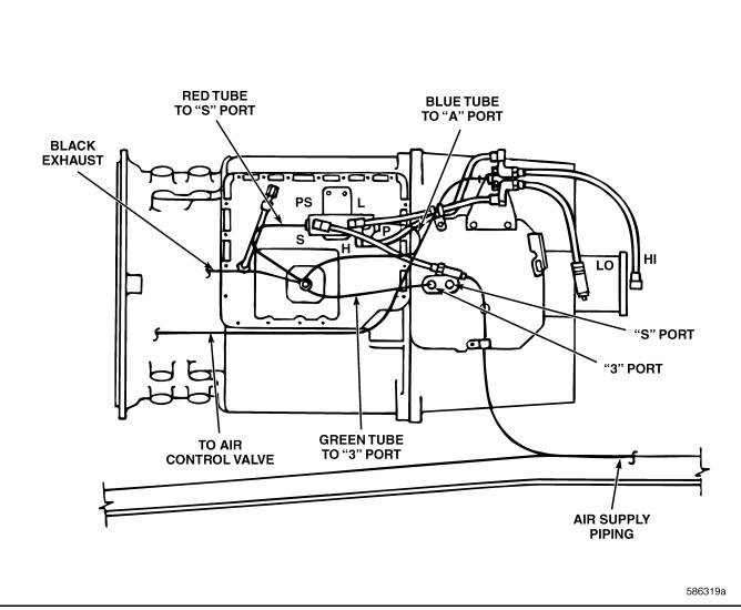
Figure 593 — Air Piping Diagram
