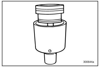
Figure 470 — Pushing Piston Assembly into Cylinder
