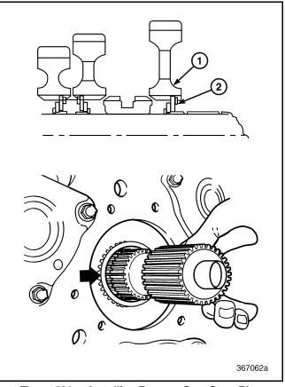
Figure 531 — Installing Reverse Gear Snap Ring (T313L/T318L Shown)
