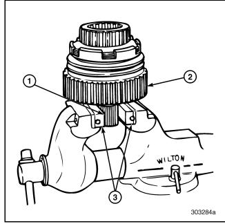
Figure 230 — Position Assembly in Soft Jaw Vise (T313L/T318L Shown)
