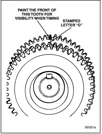
Figure 512 — Gear Tooth Marked for Timing
