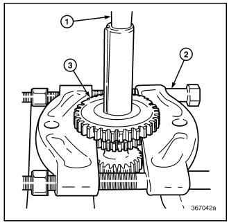
Figure 281 — Pressing First (Fifth) Gear off Shaft
