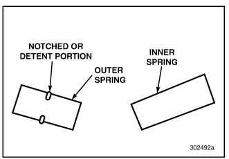
Figure 361 — Assembling Preload Springs
