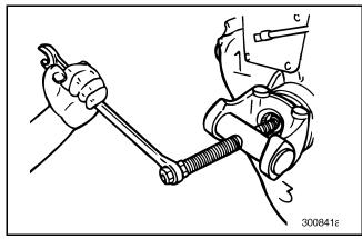
Figure 70 — Removing Drive Yoke (T313L/T318L Shown)
