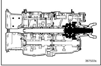
Figure 355 — Rear Mainshaft (Output Shaft) and Synchronizer Component Locator (T313L21/T318L21 Shown)
