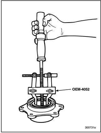
Figure 268 — Removing Bearing from Bearing Cover
