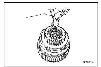
Figure 232 — Removing Larger Snap Ring in Gear (T313L/T318L Shown)
