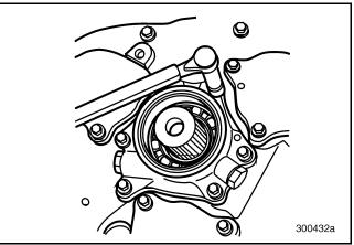
Figure 560 — Installing Rear Mainshaft Bearing Cover Assembly and Tightening Capscrews (T313LR/T318LR Shown)
