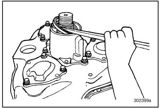
Figure 78 — Removing Output Housing Oil Seal for T313L21/T318L21 Series
