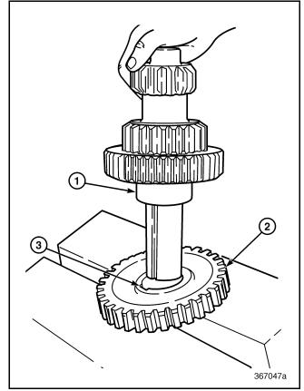
Figure 330 — Aligning Keyway with Second (Sixth) Gear
