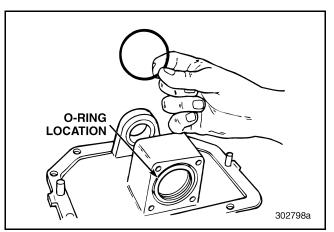
Figure 475 — Installing O-Ring onto Front of Housing
