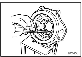
Figure 200 — Removing Bearing Cover Oil Seal
