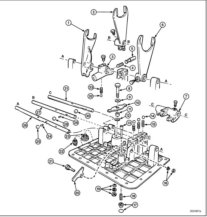
Figure 128 — Exploded View of Main Case Shift Cover
