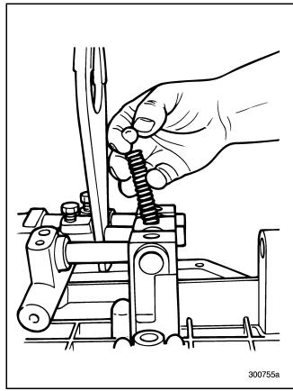
Figure 502 — Installing Poppet Ball and Spring
