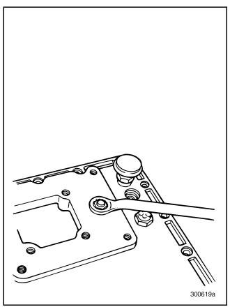
Figure 155 — Loosening Third/Fourth Rocker Pin Nut
