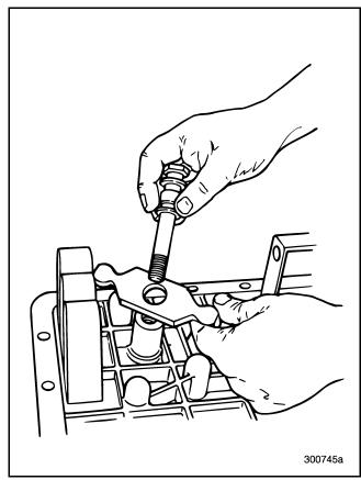
Figure 157 — Removing Third/Fourth Rocker Pin and Rocker Arm
