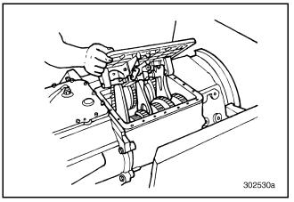
Figure 575 — Installing Main Case Shift Cover Assembly
