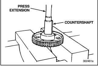
Figure 293 — Pressing off Hi-Range/Hi-Split Gear
