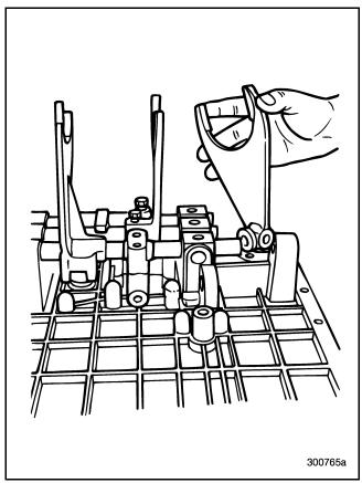
Figure 135 — Removing Lo/Reverse Shift Fork
