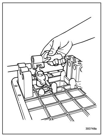
Figure 488 — Installing Shift Rail and Shifter
