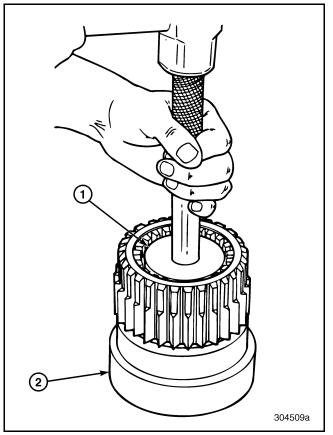
Figure 236 — Removing Ball Bearing from Gear (T313L/T318L Shown)
