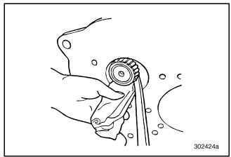
Figure 121 — Moving and Blocking No. 1 (Upper Left) Countershaft Away from Mainshaft
