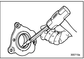
Figure 287 — Removing Front Bearing Cup
