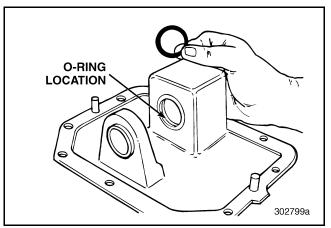
Figure 165 — Removing O-Ring from Rear of Housing
