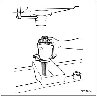
Figure 352 — Positioning Bearing Cone
