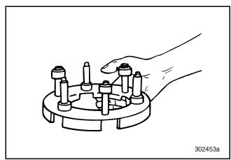
Figure 264 — Removing Synchronizer Pins
