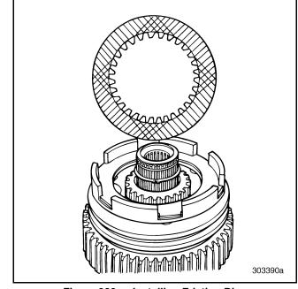
Figure 380 — Installing Friction Disc (T313L/T318L Shown)
