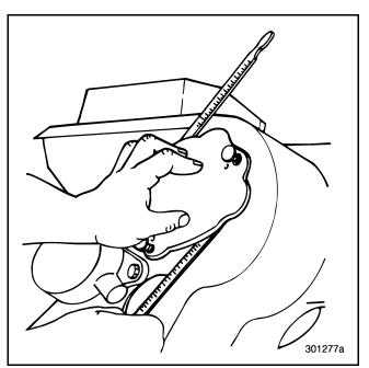
Figure 557 — Measuring with Tapered Feeler Gauges
