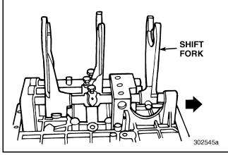
Figure 506 — Shift Rail in Position
