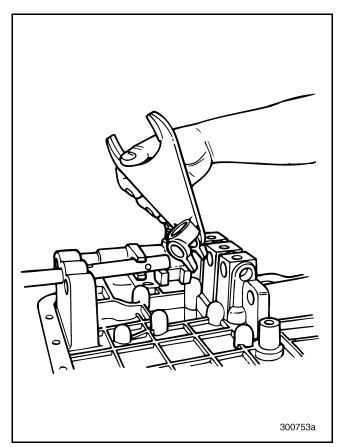
Figure 492 — Installing First/Second Shift Fork
