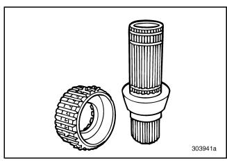
Figure 371 — Installing Lo-Range Gear Hub (T313L/T318L Shown)
