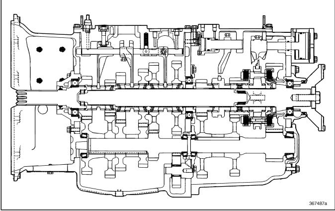
Figure 5 — Cutaway View of T313LR/T318LR Transmission
