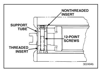
Figure 365 — Installing 12-Point Screws and Inserts
