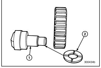
Figure 517 — Order of Reverse Idler Shaft and Components
