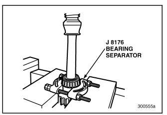
Figure 291 — Pressing off Rear Bearing Cone
