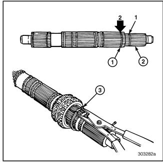
Figure 406 — Installing Second Speed Gear Mainshaft Snap Ring (T313L/T318L Shown)
