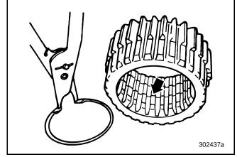
Figure 391 — Installing Snap Ring into Gear (T313L21/T318L21 Shown)
