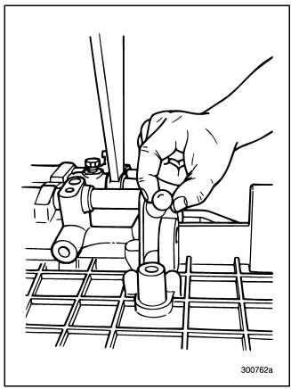
Figure 501 — Installing Interlock Ball
