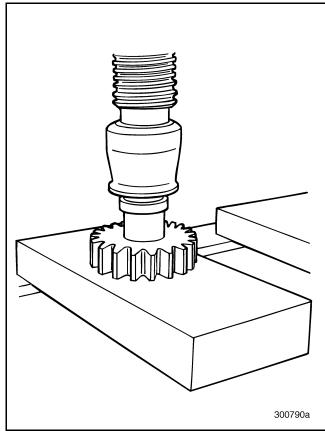
Figure 307 — Pressing Bearing into Gear
