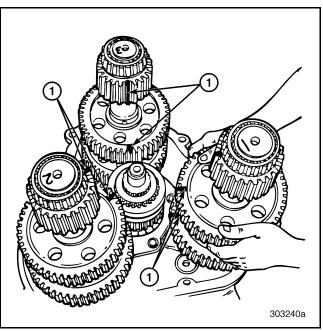
Figure 97 — Removing Compound Countershafts (T313L/T318L Shown)
