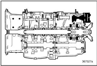
Figure 179 — Range Shift Cylinder Component Locator (T313L/T318L Shown)
