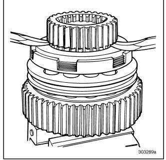
Figure 235 — Removing Hi-Range/Hi-Split Gear and Ball Bearing (T313L/T318L Shown)
