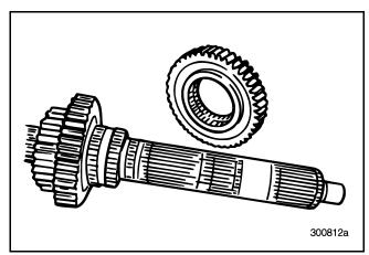
Figure 212 — Removing First Speed Gear from Mainshaft (T313L/T318L Shown)
