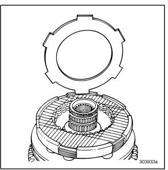
Figure 247 — Removing Reaction Disc (T313L/T318L Shown)
