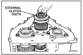
Figure 98 — Removing Splitter Sliding Clutch
