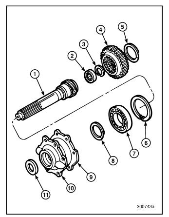
Figure 426 — Exploded View of Main Drive Pinion
