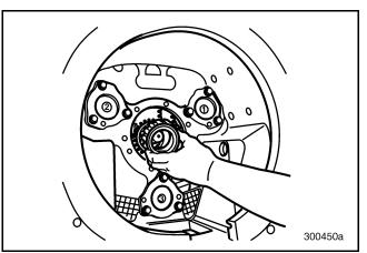
Figure 540 — Installing Sliding Clutch
