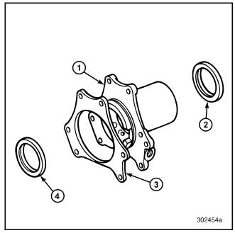
Figure 347 — Exploded View of Rear Output Housing
