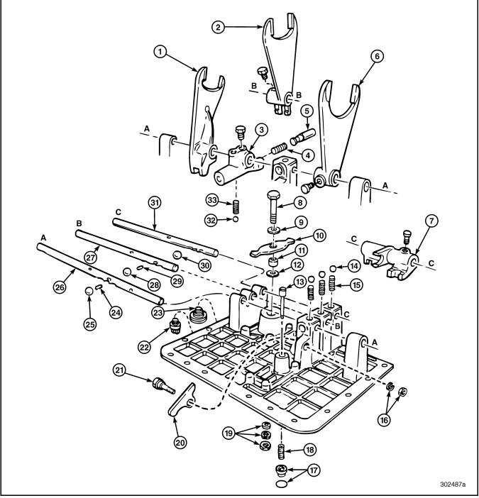
Figure 482 — Exploded View of Main Case Shift Cover
