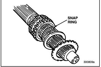
Figure 221 — Removing Second Speed Gear Externaland Internal-Toothed Thrust Washers
