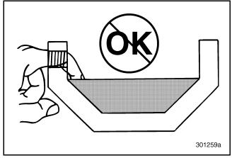
Figure 57 — Incorrect Oil Level
