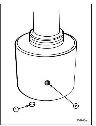
Figure 60 — Shift Cylinder Breather Vent Shown Removed (1) and Installed (2)
