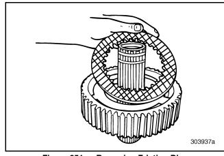
Figure 251 — Removing Friction Disc (T313L/T318L Shown)
