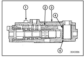
Figure 595 — Cutaway View of Range Shift Interlock Valve Assembly
