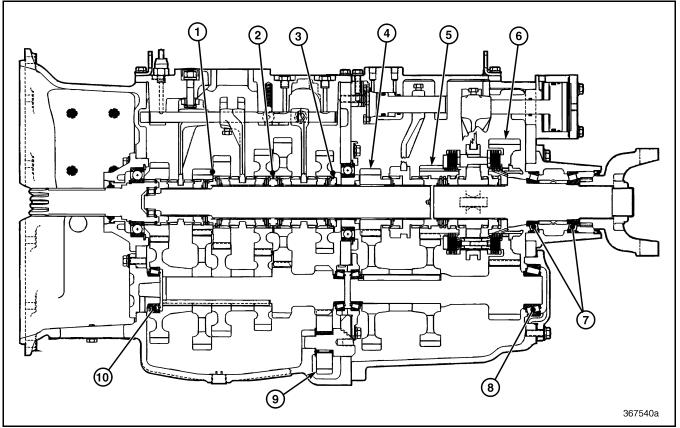
Figure 589 — Gear End Play and Bearing Preload (T313L21/T318L21 Shown)
