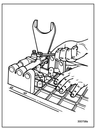
Figure 141 — Removing Setscrew from First/Second Shift Fork
