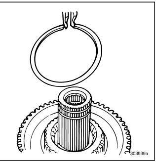
Figure 254 — Removing Gear-to-Hub Snap Ring (T313L/T318L Shown)
