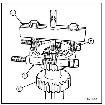
Figure 282 — Removing Rear Bearing Cone
