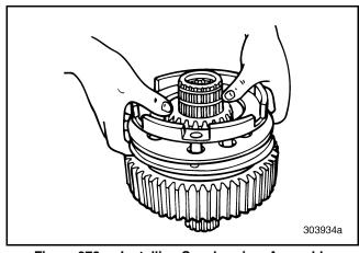
Figure 378 — Installing Synchronizer Assembly (T313L/T318L Shown)
