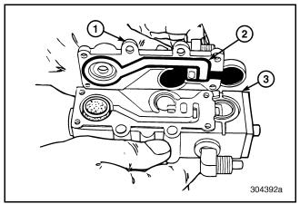
Figure 439 — Installing Top Cover Seal
