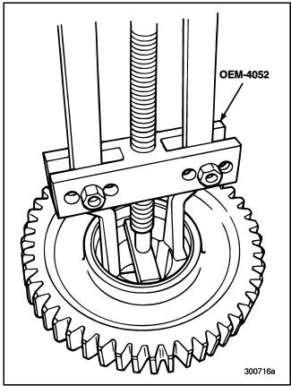
Figure 284 — Removing Bearing Cup from Main Drive Gear
