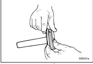
Figure 184 — Removing Teflon<sup>®</sup> Seal and O-Ring from Piston Grooves
