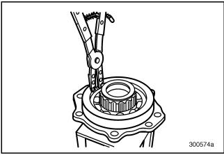
Figure 196 — Removing Main Drive Pinion Cover Bearing Snap Ring
