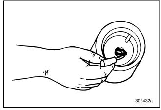
Figure 172 — Removing Shift Cylinder Inside O-Ring
