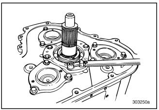
Figure 539 — Installing Front Mainshaft Rear Bearing Cover (T313L/T318L Shown)
