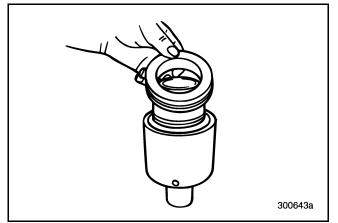
Figure 469 — Installing Sleeve onto Shift Piston
