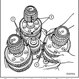
Figure 551 — Installing and Aligning Timing Marks (T313L/T318L Shown)
