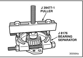
Figure 276 — Removing Bearing Cone from Front Countershaft Front Bearing Cover
