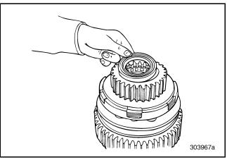
Figure 385 — Inserting Ball Bearing (T313L/T318L Shown)
