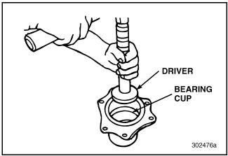
Figure 348 — Driving Bearing Cup into Output Housing
