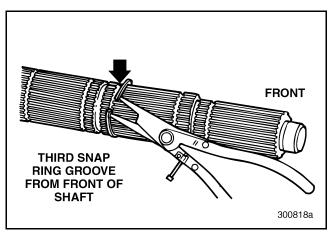
Figure 404 — Installing First Speed Gear Snap Ring
