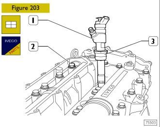
Fit a new seal (3) on the electro-injector (1) and mount this in the overhead (2).
