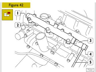
Only for forged version hydraulic accumulator, take off pipe fitting (4) and disconnect piping (5) for fuel recovery from overpressure valve (3).
