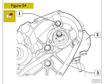
Take out the screws (1) and remove the high-pressure pump (2) from the water pump mounting (3).
