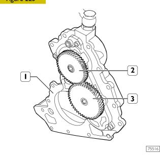
The oil pump (3) is a gear pump driven directly by the crankshaft.
