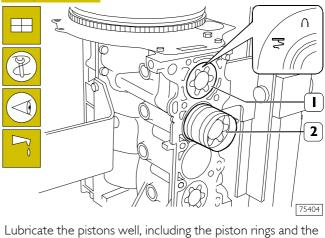
With the aid of the clamp 99360605 (2), fit the connecting
