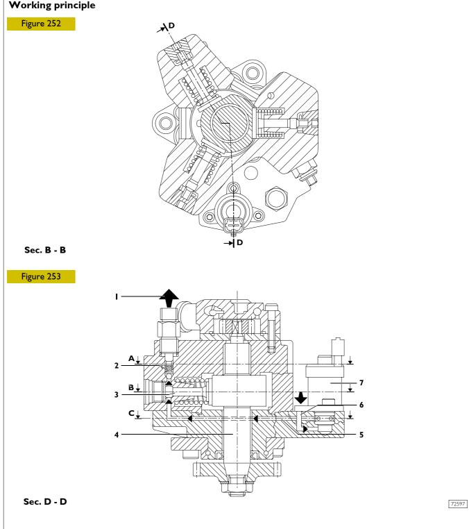
1. Outlet for delivery to rail – 2. Delivery valve to rail – 3. Pumping element – 4. Pump shaft – 5. Pumping element supply duct – 6. Pressure regulator supply duct – 7. Pressure regulator.
