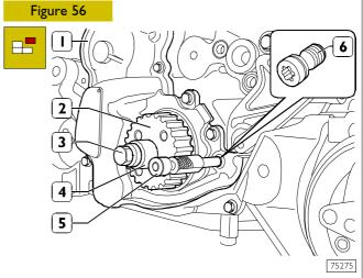
Remove the plug (6) from the oil pump - vacuum pump assembly (1).
