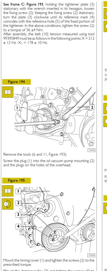
Mount the damper pulley (3) and tighten the screws (4) to the prescribed torque.
