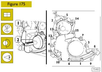
Fit the centring tool 99396037 (2) onto the shank of the crankshaft.
