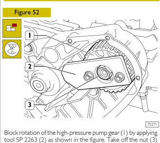
tool SP 2263 (2) as shown in the figure. Take off the nut (3 and remove the tool (2).
