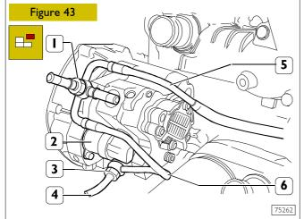
Disconnect the fuel recovery pipes (4), (5) and (6) from the high-pressure pump (2), removing the couplings (1) and (3).
