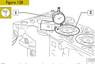
After mounting the connecting rod - piston assemblies, check the protrusion of the pistons (2) at the T.D.C. in relation to the top surface of the crankcase with a dial gauge (1).
