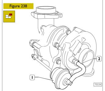
Cover the air, exhaust gas and lubricating oil inlets and outlets. Thoroughly clean the outside of the turbocharger using anticorrosive and antioxidant fluid. Disconnect the pipe (2) from the union of the pressure relief valve (1) and fit on it the pipe of the device 99367121 (1, Figure 239).
