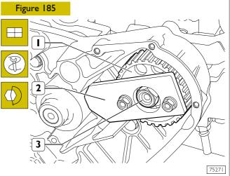
Fit the driving gear (1) onto the shaft of the high-pressure pump and block rotation of this shaft by applying tool SP.2263 (2) as illustrated in the figure. Tighten the nut (3) to the prescribed torque and remove the tool (2).
