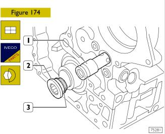
Fit the oil pressure control valve (1) in the crankcase.
