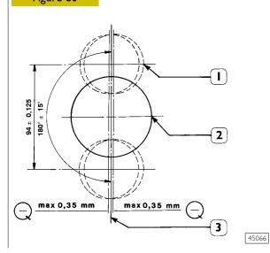
**NOTE** The checks on the tolerances indicated in the figures must be made after grinding the crankshaft pins.
