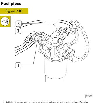
High-pressure pump supply pipe quick-coupling fitting –
