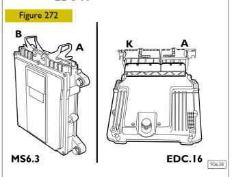
The control unit is a "flash EPROM" and so it can be reprogrammed from outside without changing the hardware. It processes the signals from the sensors by applying software algorithms and controls the actuators (especially the electro-injectors and pressure regulator).
