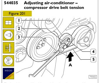
Fit the tightener (1) without tightening the screw (4). Fit the drive belt (5) taking care to position its ribs correctly in the respective races of the pulleys. With tool SP. 2341 (2) inserted in the holes of the tightener (1) and torque wrench (3), turn the tightener (1) with a torque of 8.2 - 10 Nm; in this condition, tighten the screw (4) to a torque of 25 Nm.
