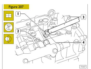
Using the wrench (4) of the 99317915 series and the torque wrench 99389829 (3), tighten the fuel pipe fittings (1) and (2) to the prescribed torque.
