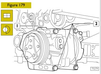
Mount the air-conditioner compressor (1) (if applicable) and tighten its fixing (2) screws to the prescribed torque.
