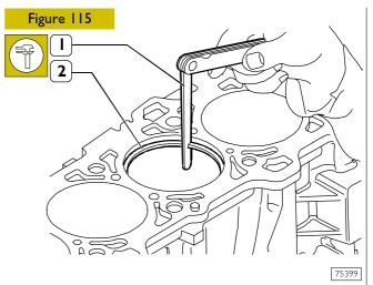
Check the opening between the ends of the piston rings (2) inserted in the cylinder liner using a feeler gauge (1).
