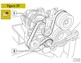
Using the specific wrench on the automatic tightener (2), slacken the tension of the belt (1) and remove it.
