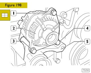
Position the alternator (2) on the mounting (5) and secure it with the bottom screws (3 and 4) and the bolt.
