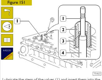
Lubricate the stem of the valves (1) and insert them into the associated valve guides (4) according to the position marked during removal. Using tool SP.2264 (2), mount the oil seals (3) on the valve guides (4).
