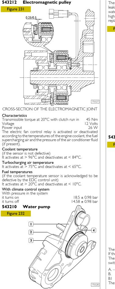
The water pump (3) cannot be overhauled. In case of coolant leaking from the seal or damage, it must be replaced. The water pump casing (1) is also used as a mounting for the high-pressure pump. The seals (3 and 4) must always be replaced.
