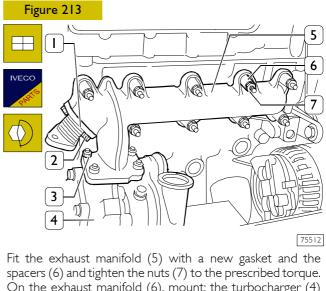
spacers (6) and tighten the nuts (7) to the prescribed torque. On the exhaust manifold (6), mount: the turbocharger (4) with a new gasket and tighten the nuts (3) with washers to the prescribed torque, the compensator pipe (1) (if applicable) with a new seal and tighten the nuts (2) with washers to the prescribed torque.
