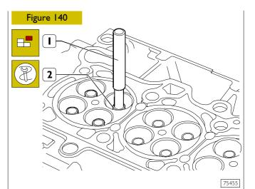
Remove the valve guides (2) with the drift SP.2312 (1).
