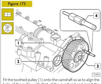
Fit the toothed pulley (1) onto the camshaft so as to align the hole of the pulley with that of the overhead and insert the tool 99360608 (4) into these holes. Screw down the screw (3) together with the washer (2) without tightening fully.
