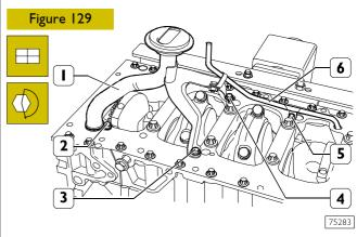
Mount the suction strainer (1) together with the pipe (6). Screw down the fixing screws (2-3-4-6) and tighten them to the prescribed torque.
