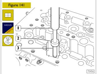
Heat the cylinder head to  $80 - 100^{\circ}$ C and, using the drift SP.2312 (1) provided with part SP.2311 (2), mount the new valve guides (3) previously chilled in liquid nitrogen.
