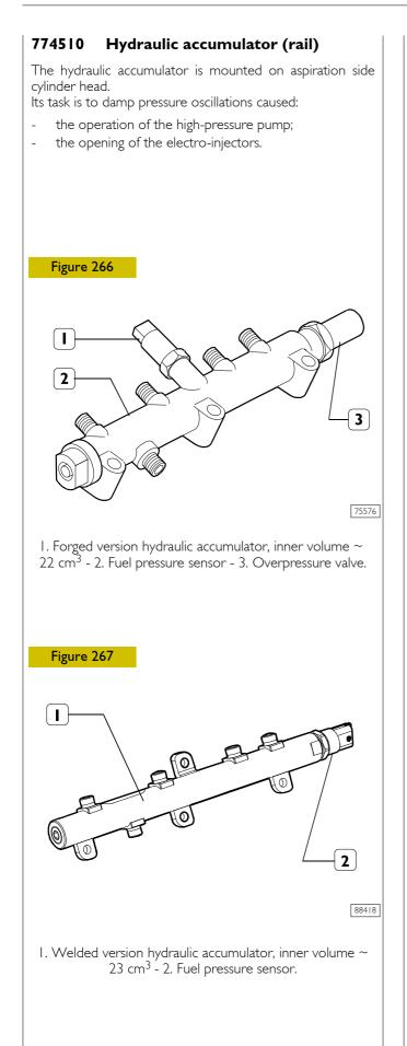
Overpressure valve (for forged hydraulic accumulator)
