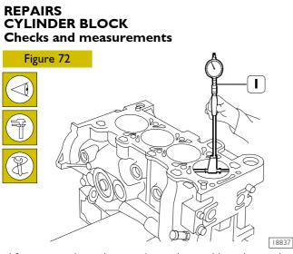
After removing the engine, thoroughly clean the cylinder-crankcase assembly. Use the rings 99365508 to carry the cylinder block.
