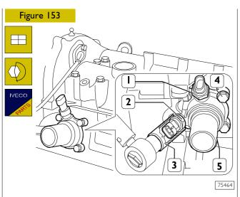
Fit the thermostat casing (5) with a new seal and tighten the fixing screws (4) to the prescribed torque.
