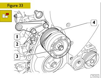
Take out the screws (2) and (3) and remove the mounting (1) together with the electromagnetic coupling (4).
