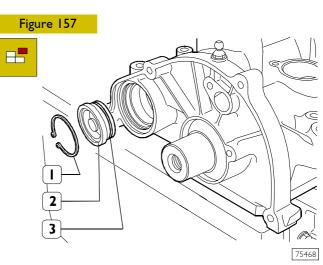
Remove the circlip (1) and take off the cover (2) together with the seal (3).
