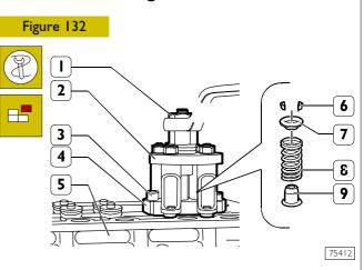
Fit part (4) of tool 99360260 onto the cylinder head (5) and secure it with the screws (3).
