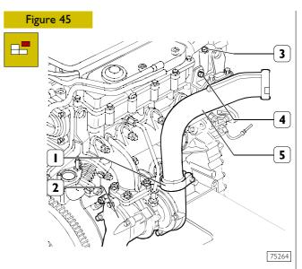
Take out the screw (4), loosen the clamp (1) and disconnect the air duct (5) from the turbocharger (2) and from the overhead (3).
