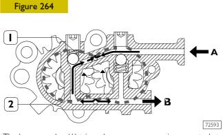
The by-pass valve (1) trips when overpressure is generated at the outlet B. The pressure, overcoming the elastic resistance of the spring of the valve (1), sets the outlet in communication with the inlet via the duct (2).
