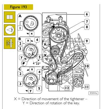
Turn the automatic tightener (1) clockwise, positioning it as shown in frame A.
