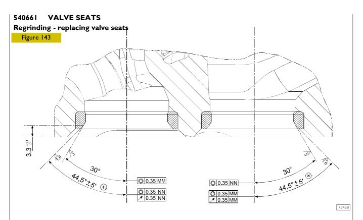
Check the valve seats. On finding any slight scoring or burns, regrind them with an appropriate tool according to the angles given in Figure 143.
