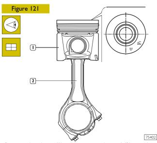
Connect the piston (1) to the connecting rod (2) together with its cap so that the piston assembly reference, position of the connecting rod and of the cap are observed as shown in the figure.
