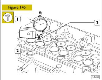
Using a dial gauge (1), check that, from the plane of the cylinder head, the valve recessing (2) and the protrusion of the injector (3) and of the glow plug have the prescribed value:
