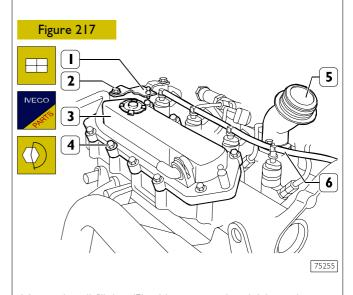
Mount the oil fillpipe (5) with a new seal and tighten the nuts (6) to the prescribed torque.
