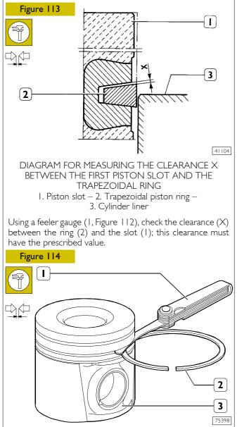
Check the clearance between the piston rings (2) of the  $2^{nd}$  and  $3^{rd}$  slot and the associated seats on the piston (3) with a feeler gauge (1).
