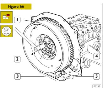
Block rotation of the flywheel (1) with tool 99360306 (3). Take out the screws (2) and remove the engine flywheel (1). Take out the screw (5) and remove the guard (4).
