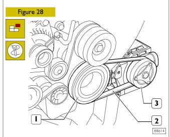
Or, on the engines with elastic belt (2), with a suitable tool, take the belt off pulleys (1 and 3).
