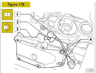
Mount the speed sensor (1) with a fresh gasket and tighten the fixing screw (2) to the prescribed torque (if applicable).
