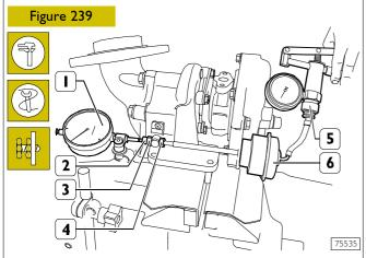
Rest the tip of the dial gauge (1) with a magnetic base on the end of the tie rod (2) and zero it. Using the device 99367121 (5), introduce compressed air into the valve casing (6) at the prescribed pressure and make sure this value stays constant throughout the check; replace the valve if it doesn't. In the above conditions, the tie rod must have made the prescribed travel. On finding a different value, use the nuts (3 and 4).
