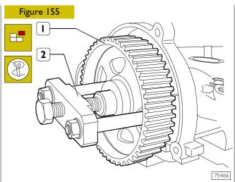
Using the extractor 99340028 (2) extract the toothed pulley (1) driving the camshaft.
