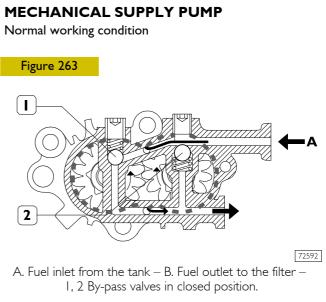
The function of the gear pump, mounted on the rear of the high-pressure pump, is to supply the high-pressure pump. It is governed by the shaft of the high-pressure pump. In normal working conditions, the flow of fuel inside the mechanical pump is shown in the figure.
