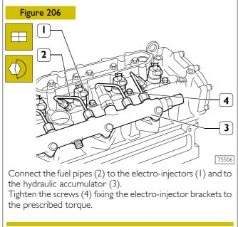
**NOTE** Whenever they get removed, the fuel pipes must be replaced with new ones.
