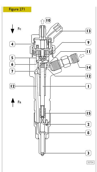
I Pressure rod – 2 Pin – 3 Nozzle – 4 Coil – 5 Pilot valve –
