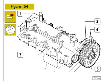
Position the overhead (2) together with the pins 99360614 (1) on the mounting SP. 2271.
