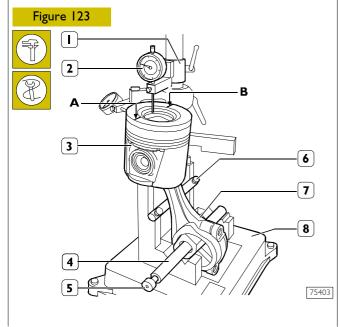
After fitting the connecting rod – piston assembly together, check for distortion with the tool 99395363 (8) as follows:
