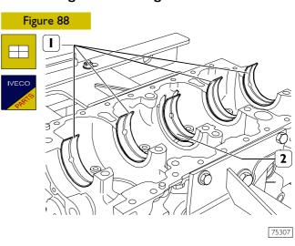
**NOTE** Not having found it necessary to replace the main bearings, they need to be fitted back on in the same sequence and position found upon disassembly.
