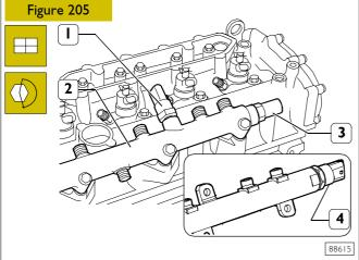
Forged version: on hydraulic accumulator (2), mount: pressure sensor (1) tightening it at  $35 \pm 5$  Nm torque, and pressure relief valve (3) tightening it at  $27 \pm 2$  Nm torque. Welded version: mount pressure sensor and tighten it at 70  $\pm 5$  Nm torque.
