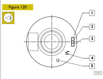
Etched on the top of the piston are: the type of engine (1), class selection (2) and supplier (3) as well as the direction of fitting the piston in the cylinder liner (4). The mark (5) is for passing the  $1^{st}$  slot insert adhesion test.
