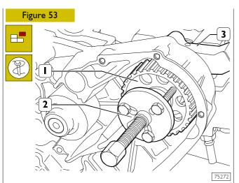
Using tool 99340035 (2), applied as in the figure, extract the gear (1) from the shaft of the high-pressure pump (3).
