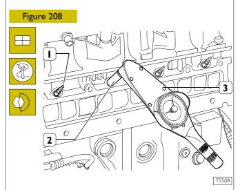
Mount the glow plugs (1) and, using the box-type wrench SP. 2275 (2) and torque wrench 99389819 (3), tighten them to a torque of 8  $\div$  10 Nm.
