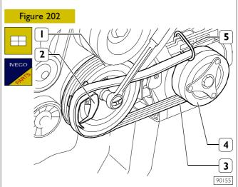
Fit the flexible belt (3) equipped with tool 99360191 (2) on the pulley (4) and apply the tool on the pulley (1). Fit the drive ring (5) on the flexible belt (3) and fasten the ring on the compressor support.
