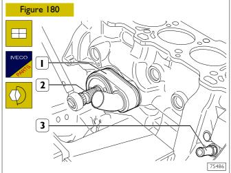
Mount the oil pressure transmitter (3) with a fresh gasket.
