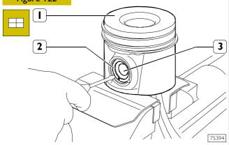
Position the piston (1) on the connecting rod, insert the pin (3) and secure it with the split rings (2).
