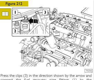
connect the fuel recovery pipe fittings (1) to the electro-injectors (2).
