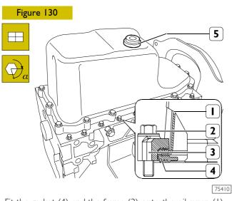
Fit the gasket (4) and the frame (3) onto the oil sump (1). Screw down the fixing screws (2) and tighten them to the prescribed torque.
