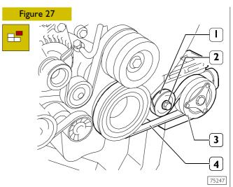
Take off screw (2), if present, and dismount belt tensioner (1). Take off the belt (4) driving the air-conditioner compressor (3).
