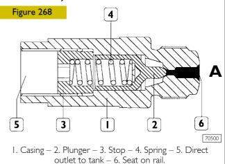
The pressure relief valve protects the system components if the fuel pressure exceeds the setting: 1750 bars.
