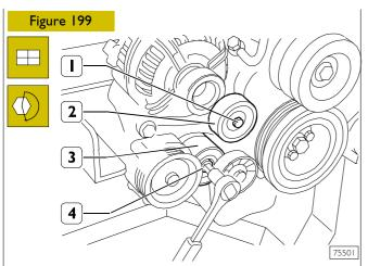
Mount the fixed tightener (2) and tighten the fixing screw (1).
