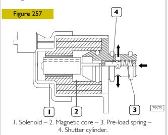
When the solenoid (1) is not energized, the magnetic core is pushed into the rest position by the pre-load spring (3). In this condition, the shutter cylinder (4) is in such a position as to offer the fuel the greatest section of passage.
