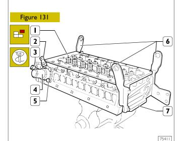
Place the cylinder head (1) on the mounting SP.2271 (7). Remove the brackets (6) for lifting the engine.
