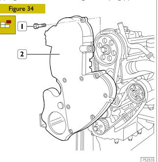
Take out the screws (1) and remove the timing cover (2).
