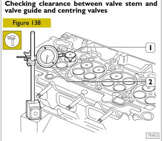
The checks are made using a dial gauge (2) with a magnetic base, positioned as illustrated. The assembly clearance is 0.033 - 0.063 mm.
