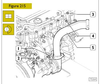
Connect the air duct (5) to the turbocharger (2) and to the overhead (3).
