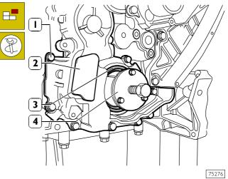
Apply tool 99340057 (4) to the front O-ring (3) of the crankshaft and remove it from the oil pump – vacuum pump assembly (2).
