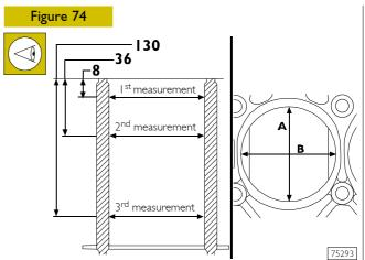
The measurements must be made for each single cylinder at three different heights up the liner and on two planes at right angles to each other: one parallel to the longitudinal axis of the engine (B) and the perpendicular (A); the greatest wear is generally found on this last plane with the first measurement.
