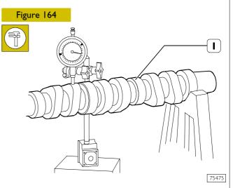
Set the shaft (1) on tailstocks and, using a dial gauge on the middle mounting, check that the alignment error is no greater than 0.04 mm; replace the shaft if it is. In addition, check the cam lift: it must be as prescribed; replace the shaft if it is any different.
