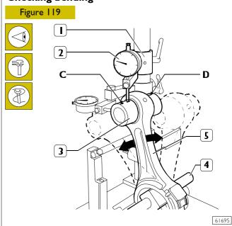
Check the bending of the connecting rod (5) by comparing two points C and D of the pin (3) on the vertical plane of the axis of the connecting rod.
