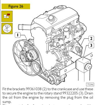
Disconnect the fan from the electromagnetic coupling (1).
