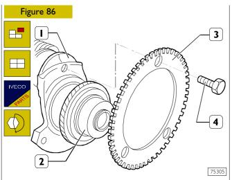
Take out the screws (4) and replace the phonic wheel (3). The screws (4) are coated with LOCTITE 218 and must be replaced with fresh ones after each disassembly. They must be tightened to a torque of 15 Nm.
