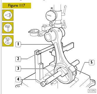
Check the alignment of the axes of the connecting rods (1) with device 99395363 (5), proceeding as follows:
