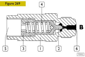
B. If the pressure of the fuel in the hydraulic accumulator exceeds 1750 bars, the plunger gets shifted and the excess pressure is discharged into the tank.
