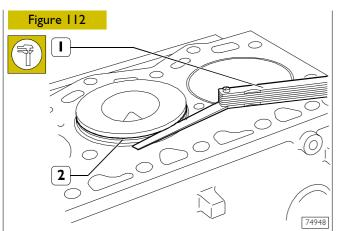
Check the clearance between the trapezoidal ring (2) ( $1^{st}$  slot) and the associated slot on the piston with a feeler gauge (1), proceeding as follows: insert the piston into the cylinder liner so that the ring (2) comes approximately half way out of it.
