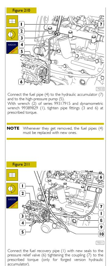
Connect the fuel recovery pipes (1) and (5) with new seals to the high-pressure pump (2) with the couplings (3) and (4). Insert the oil dipstick tube (9) with a new seal into the crankcase and secure it together with the pipe (10), using the screw (8) tightened to the prescribed torque, to the intake manifold.
