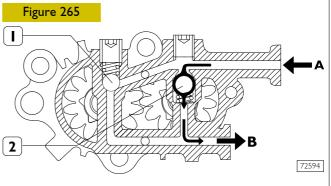
The by-pass valve (1) trips when, with the engine switched off, you want to fill the supply system via the priming pump. In this situation, the by-pass valve (2) opens, due to the effect of the inlet pressure, and the fuel flows out via the outlet B.
