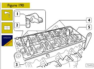
Thoroughly clean the hydraulic tappets (2), lubricate them and fit them in the cylinder head (3), positioning the rocker arms (1) on the valves correctly.
