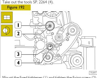
Mount the fixed tightener (1) and tighten the fixing screw (2) to the prescribed torque.
