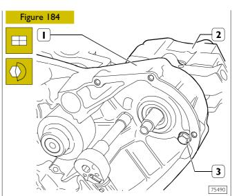
Fit the high-pressure pump (2) onto the flange of the water pump (1) and tighten the fixing screws (3) to the prescribed torque.
