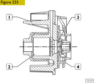
LONGITUDINAL CROSS-SECTION OF THE WATER PUMP I. Pump casing – 2. Pump drive shaft together with bearing – 3. Seal – 4. Impeller.
