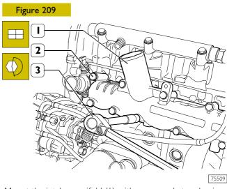
Mount the intake manifold (1) with a new gasket and, using a torque wrench (3), tighten the fixing screws (2) to the prescribed torque.
