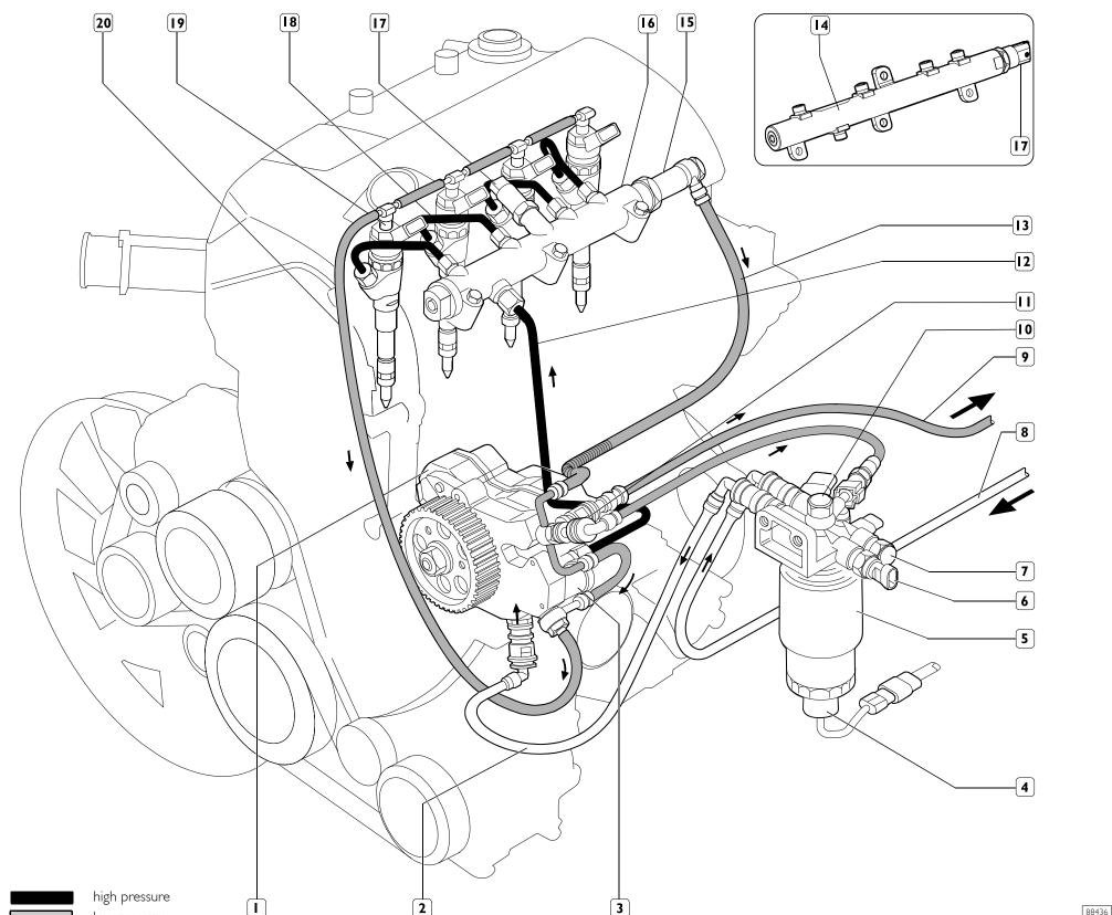
FUEL RECIRCULATION AND SUPPLY SYSTEM DIAGRAM
