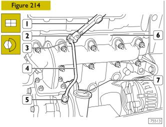
Connect the pipe (4) to the cylinder head (6) and to the turbocharger (7).
