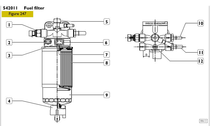
I. Clogging signalling sensor - 2. Temperature sensor connector - 3. Heater support - 4. Water in signalling sensor - 5. Overpressure valve - 6. Heater connector - 7. Bending insert - 8. Fuel filter - 9. Water separator - 10. Connector -
