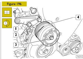
Fit on the mounting (1) together with the electromagnetic coupling (4) and tighten the fixing screws (2 and 3) to the prescribed torque.
