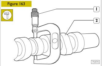
Using a micrometer (1), measure the diameter of the pins (2) of the camshaft and, using a bore meter, measure the diameter of the supporting seats in the overhead.
