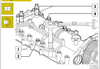
Mount the overhead (1) together with the tools 99360614 (3) for the timing and tighten the fixing screws (2) to the prescribed torque.
