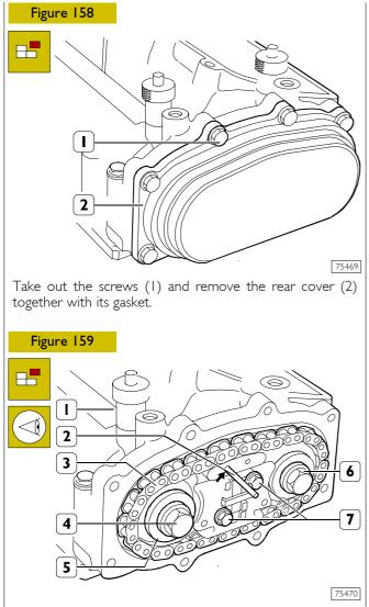
Insert a suitable pin (2) in the hole ( $\Rightarrow$ ) of the chain drive (3). Take out the screws (4) and (6) with their washers (5) for fixing gears to the camshafts.
