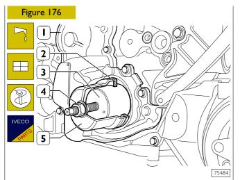
Lubricate the shank of the crankshaft.
