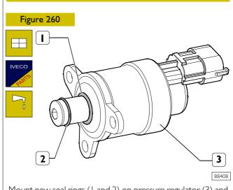
Mount new seal rings (1 and 2) on pressure regulator (3) and lubricate the rings with vaseline.
