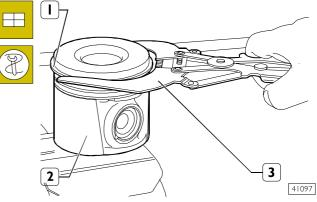
Fit the piston rings (1) on the piston (2) using the pliers 99360183 (3).
