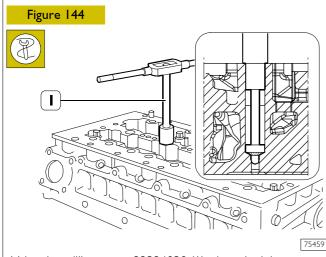
Using the milling cutter 99394038 (1), clean the injector seat of any deposits.
