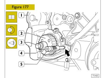
Turn the crankshaft so as to be able to insert tool 99360615 (5) into the hole in the crank of the crankshaft, through the hole in the oil vacuum pump assembly (1), to block crankshaft rotation.
