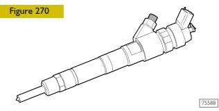
The electro-injectors have high-pressure supply (up to 1600 bar) and recirculation at atmospheric pressure, necessary for the diesel used to operate the pilot valve.
