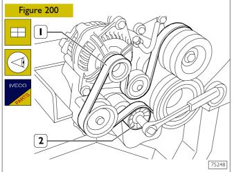
Using a wrench on the automatic tightener (2), mount the drive belt (1), taking care to position its ribs correctly in the respective races of the pulleys.
