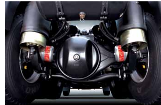
Automatic (ECAS) 4-bag type air-suspension
