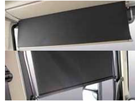
Roll-screen type sun visor (Front: Automatic, Side: Manual)
