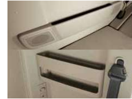
Back panel console and bedside console
