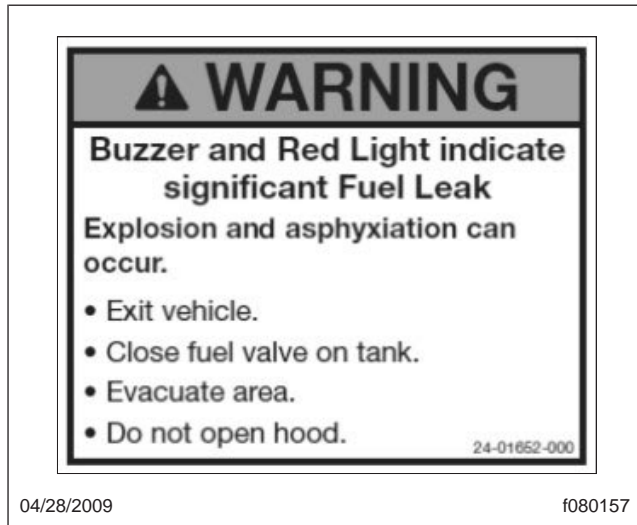
Fig. 16.4, Interior Warning Sticker
