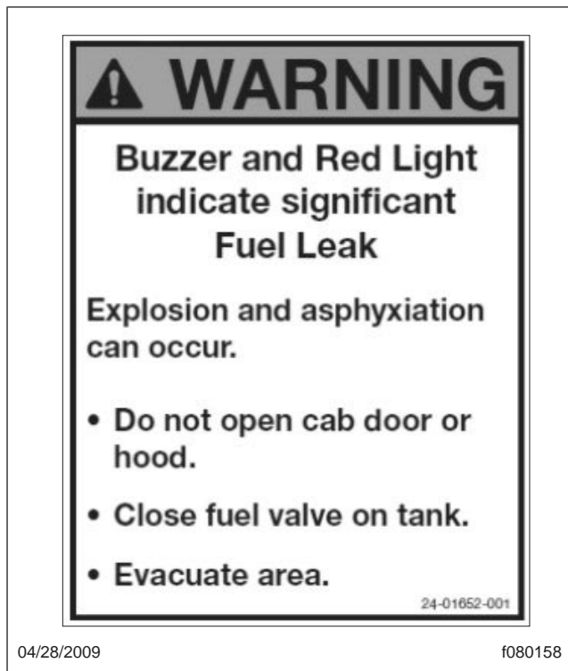
Fig. 16.5, Exterior Warning Sticker
