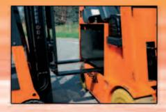
BATTERY To increase autonomy of work there are several different batteries of various amperage available. The battery, which can be removed from the vehicle laterally, can be replaced using a hoist or using another forklift. Power rating 96V.
