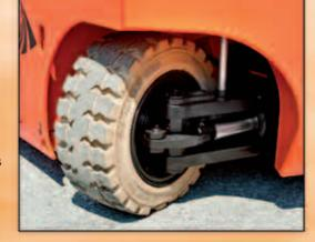
**TYRES** The Z60KN, Z65KN, Z70KN and Z80KN model uses super-elastic tyres but it can also uses cushion type tyres.
